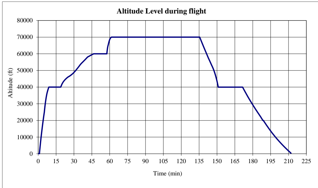
Figure 122 Line Plot of Altitude Level Variation with Respect to Time of Flight for Fixed 45° Sweep Aircraft with Maximum Weight of 675,000 lbm.
