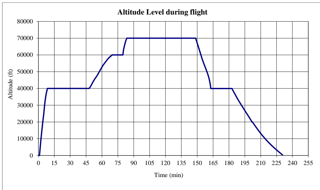
Figure 117 Line Plot of Altitude Level Variation with Respect to Time of Flight for Fixed 35° Sweep Aircraft with Maximum Weight of 675,000 lbm.
