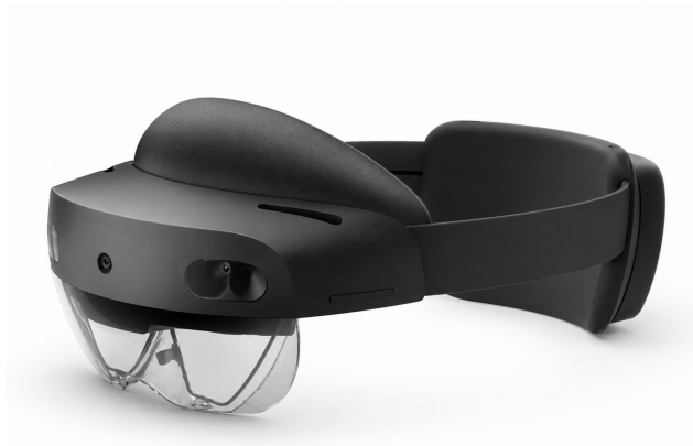
Figure 6.1: Microsoft HoloLens 2 head-mounted display used as the augmented reality endpoint. The integrated eye tracker streams gaze origin and direction at 30 Hz alongside the head pose at 60 Hz; both streams are timestamped against the same ROS2 clock as the 500 Hz admittance control loop, so saccade events and kinematic transitions can be aligned at the trial level.
