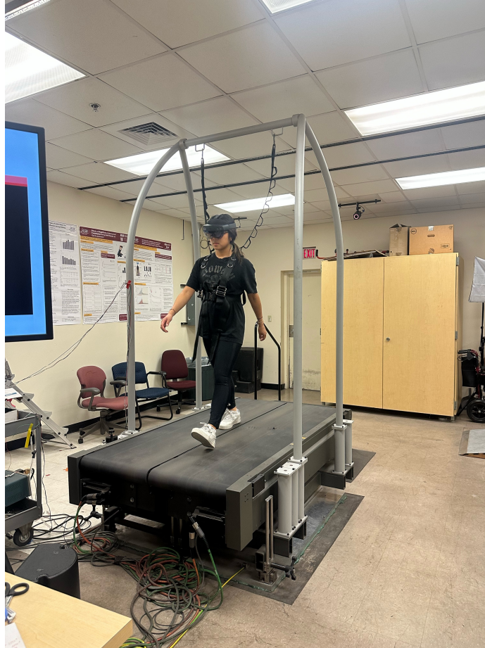
Figure 5.1: Experimental setup showing the instrumented split-belt treadmill with safety harness and motion capture markers. Visual feedback is provided via a traditional computer monitor or a Microsoft HoloLens augmented reality head-mounted display.
