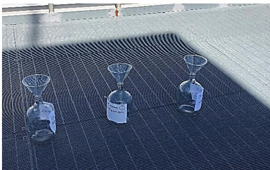
Figure B2. Deposition Samplers deployed on the rooftop of the Interdisciplinary Science & Technology Building #4 (ISTB4), ASU, Tempe
