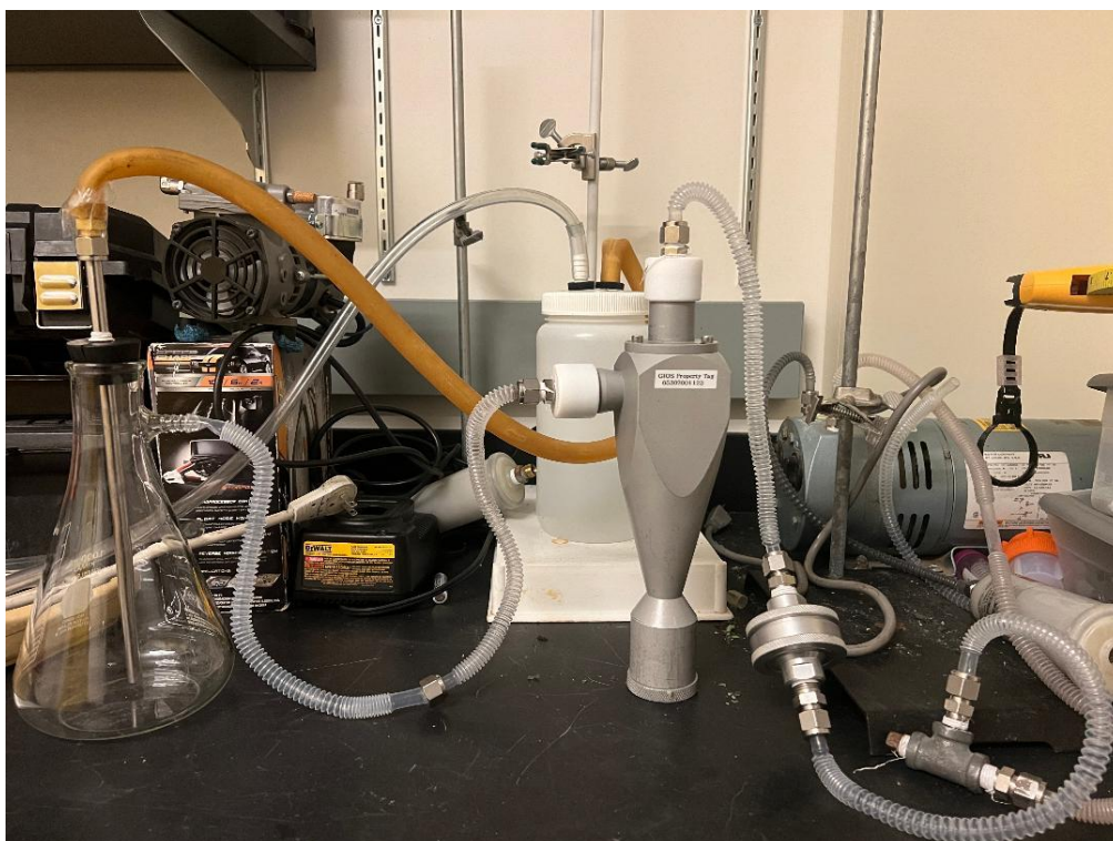
Figure D1. Resuspension setup in the laboratory to obtain PM 10 tire wear samples.
