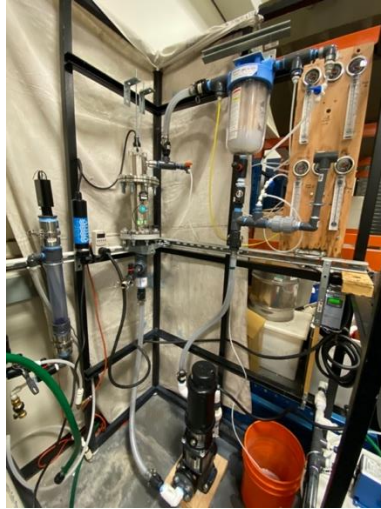
Figure 3.3 Slurry Photoreactor (Testbed Setup)
