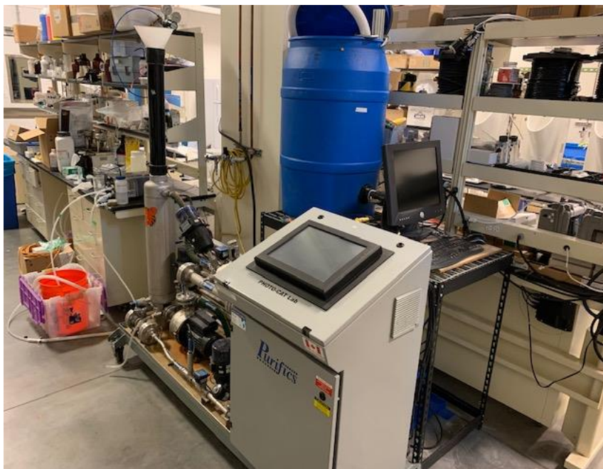
Figure 3.4 Photo-Cat from Purifics (Pilot-Scale Setup)
