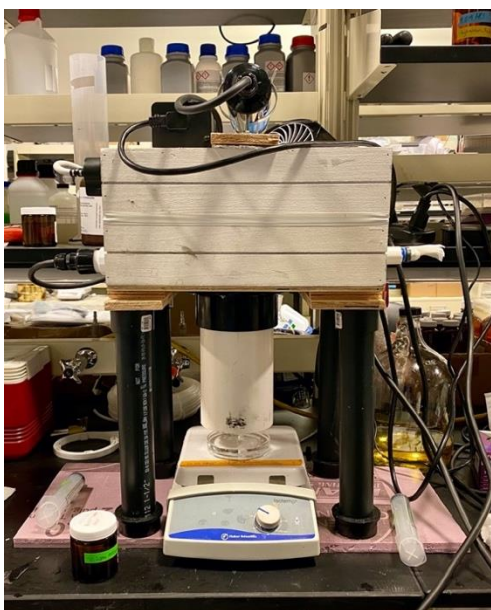
Figure 3.1 Collimated Beam (Bench-Scale Setup)
