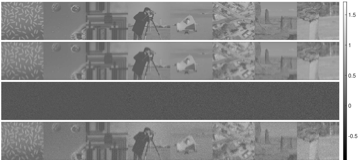
Figure 6.3: 1D validation data formed by reformatting the MATLAB ® built-in images from fig. 6.2. Each column was blurred using a Gaussian kernel with \xi = 16 . White noise was added to produce a specific SNR (in this case, an SNR of 10). The resulting vectors are shown at the bottom. The dimension of all four images is 256 \times 2,048 .
