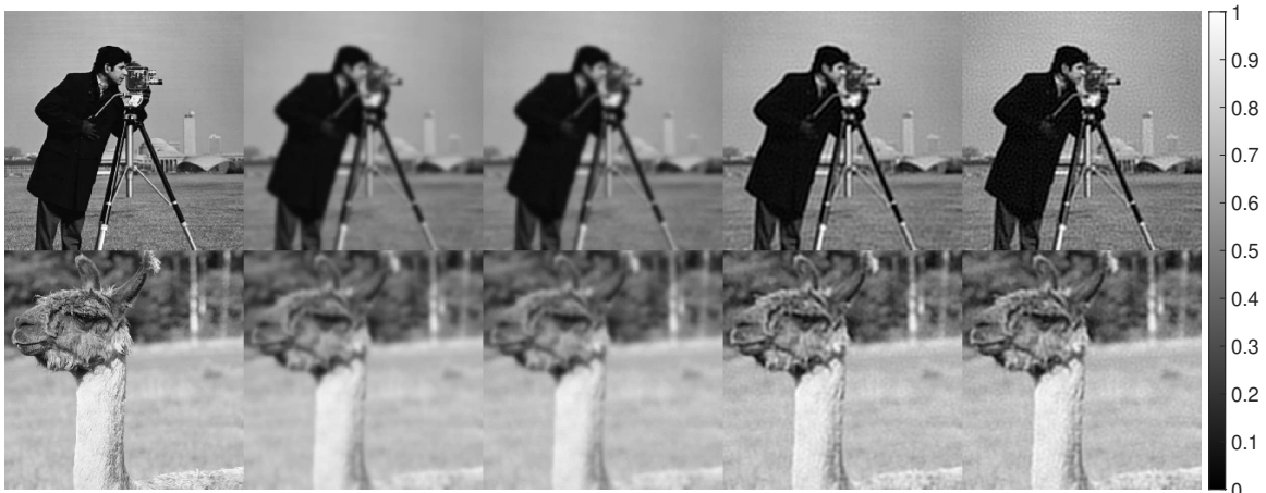
Figure 6.17: Two samples from the second validation set, with \xi = 16 , an SNR of 40, two log windows and the Laplacian penalty matrix. From left to right for each sample are the true solution, the blurred image, the blurred image after noise was added, the regularized solution obtained using the multidata windowed MDP method ( \epsilon = 1 ) with R = 8 (the entire training set), and the regularized solutions using parameters that are optimal for the individual image. The multidata windowed MDP solutions have relative errors of 10.43% and 7.09% for the top and bottom samples, respectively.
