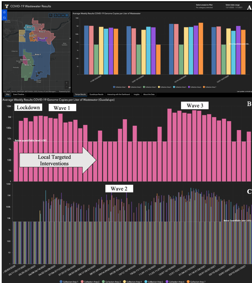
Figure 11. Publicly accessible, interactive WBE online dashboard showcasing (A) a Map of Tempe, Arizona divided into wastewater catchments (Areas 1-7 and Town of Guadalupe) alongside one month of SARS-CoV-2 levels in wastewater determined by targeting the E gene, with additional data being displayed for (B) The Town of Guadalupe (May 2020 through March 2020); with local targeted interventions implemented from May 2020 through August 2020 and (C) The City of Tempe (May 2020 through March 2020), showing the impact of the initial lockdown, and subsequent waves of infection over time (viewable at covid19.tempe.gov).
