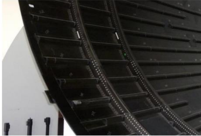
Figure 6: BOEING 787 FUSELAGE w/ RIVETED RIBS & SKINS all in composite [40]
