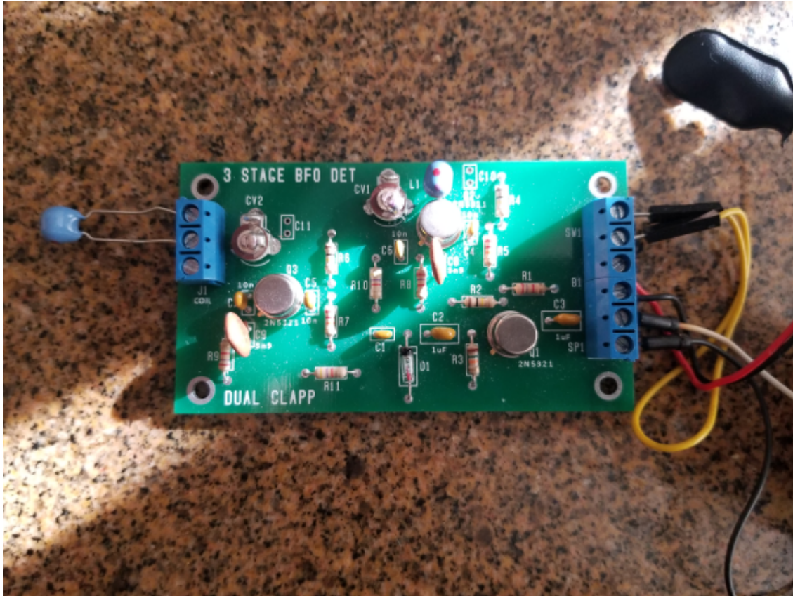
Figure 5.3: Three Stage Beat Frequency Oscillator Circuit Used for the Experiment
