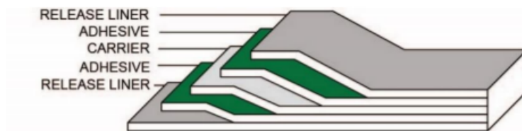
Figure 5.24: Different Layers of AR 90445Q Spacer Tape Adhesive. From Adhesives Research Inc (2020)
