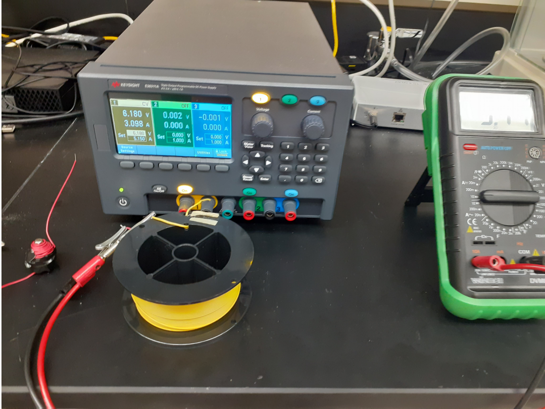
Figure 5.1: Experimental Setup Showing Supply Voltage as 6.18 Volts and Current as 3.56 Amperes
