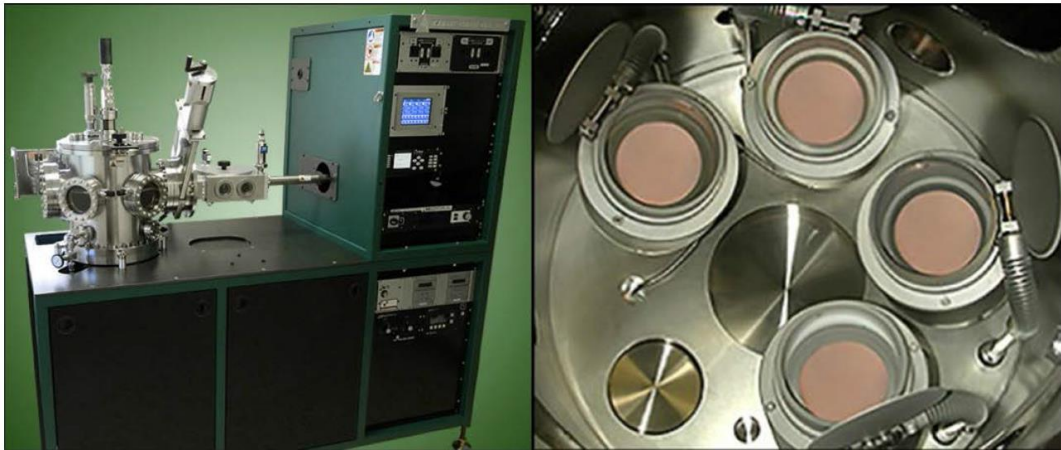
Figure 10: (left) Orion 5 Sputter Deposition Tool used to synthesize metallic films. (right) Magnetron sputtering guns having copper targets. Pictures courtesy of AJA International.
