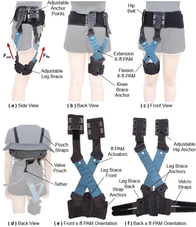
Figure 1: The SR-HExo Shown on a User from (a) the Side Profile, (b) Back View, (c) Front View, and (d) Back View. The Actuator Anchor Points and Adjustable Leg Brace in (a) Are Highly Modular to Fit Many Users. The X-ff-PAM Used for Actuation in Flexion (e) and in Extension (f) Including the Modular Knee Anchor Point
