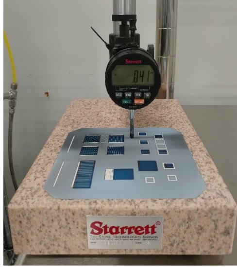
Figure 12: The Thickness of the Wafers Was Measured after Texturing, at Five Different Points, Using a Digital Thickness Gauge with 1 \mu\text{m} Resolution. Photo Shows the Measurement Tool.
