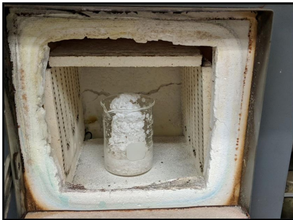
Figure B2. Transformation of gel to foamy powders on introducing into a preheated furnace held at 500 °C.
