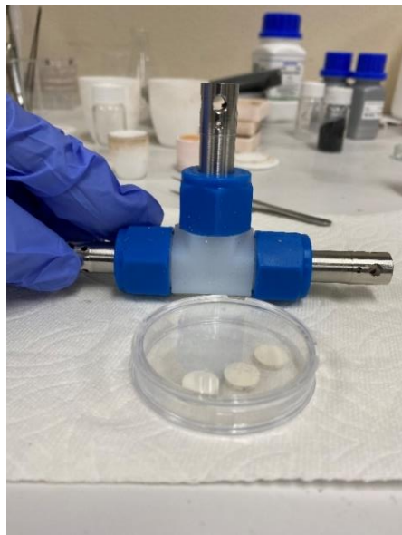
Figure 6. 2. In-house fabricated Swagelok type cell for Li||LLZO||Li cycling.
