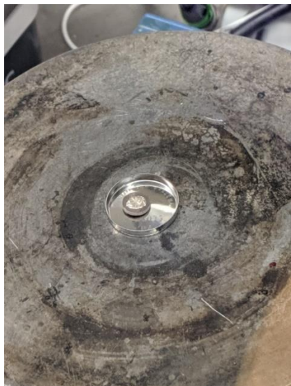
Figure 6. 1. Li metal reacting with graphite interlayer to form Li-C based interface.
