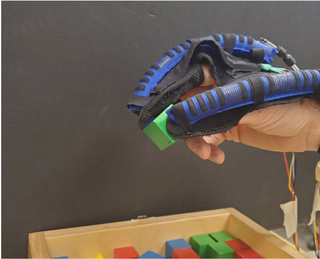
Figure B.1: Close Up of Three Finger Pinch From Box and Blocks Test
