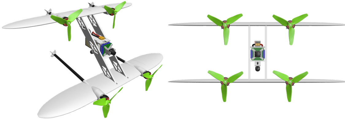
Figure 5 - Front left Isometric View (left), Front View (right) of first Iteration
