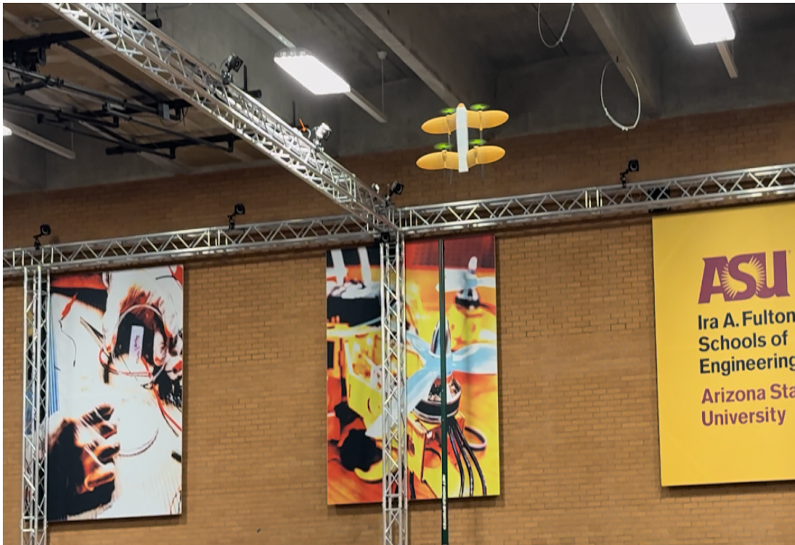
Figure 30: Aircraft Maintaining Stable Hover During Indoor Testing
