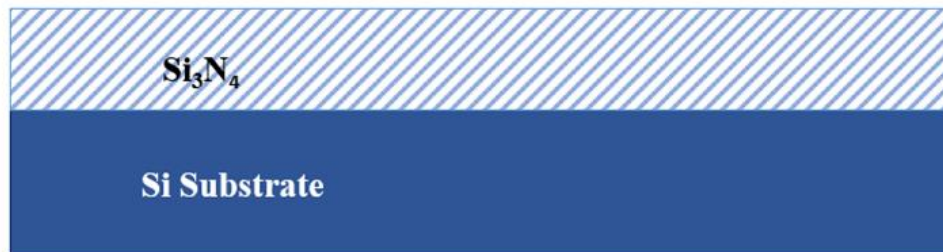
Figure 8. LPCVD deposition of \text{Si}_3\text{N}_4 .
