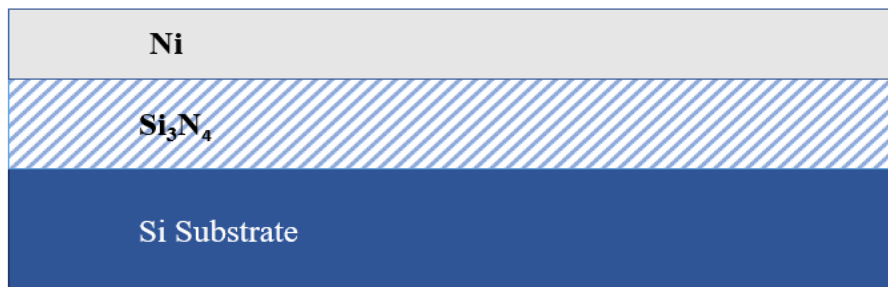
Figure 9. Deposition of Cathode (Ni) metal.
