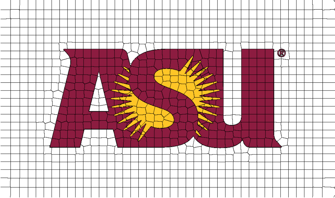
Figure 4.1: Superpixels Generated in the Custom Image Using the SLIC Algorithm.
