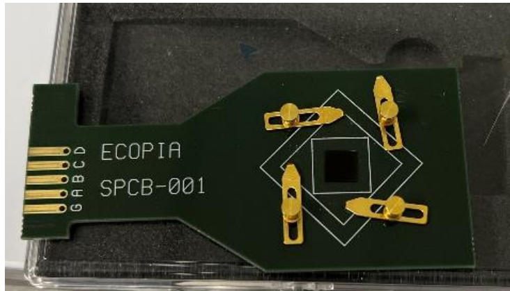
Figure 2.3.1: ECOPIA SPCB-001 testing mount for Hall effect measurements
