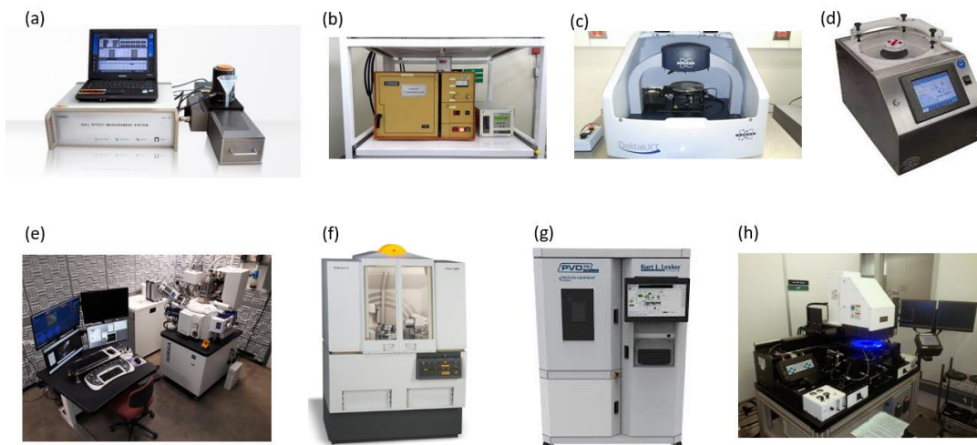
Figure 1.3.2: Images of some tools used: (a) Hall effect system (b) Barrel asher (c) Dektak profilometer (d) spin coater (e) SEM setup (f) X-ray diffractometer (g) E-beam evaporator (h) Photolithography aligner
