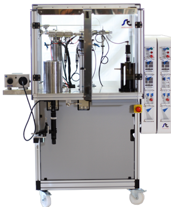
Figure 2.6: Sanchez GLS 1500 system I utilized for loading pure \text{H}_2 gas in diamond anvil cells. Image from corelab/sanchez technologies.
