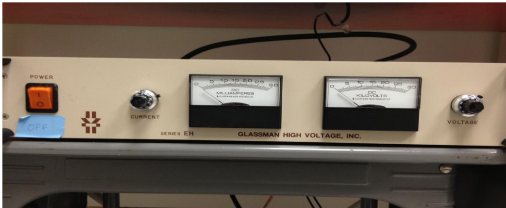
Figure 8: Shows the power supply used to supply the voltage for the electric field to spin the fibers across the air gap. The current dial was set at 1 at all times during spinning, while the voltage dial was used to control the voltage output.
