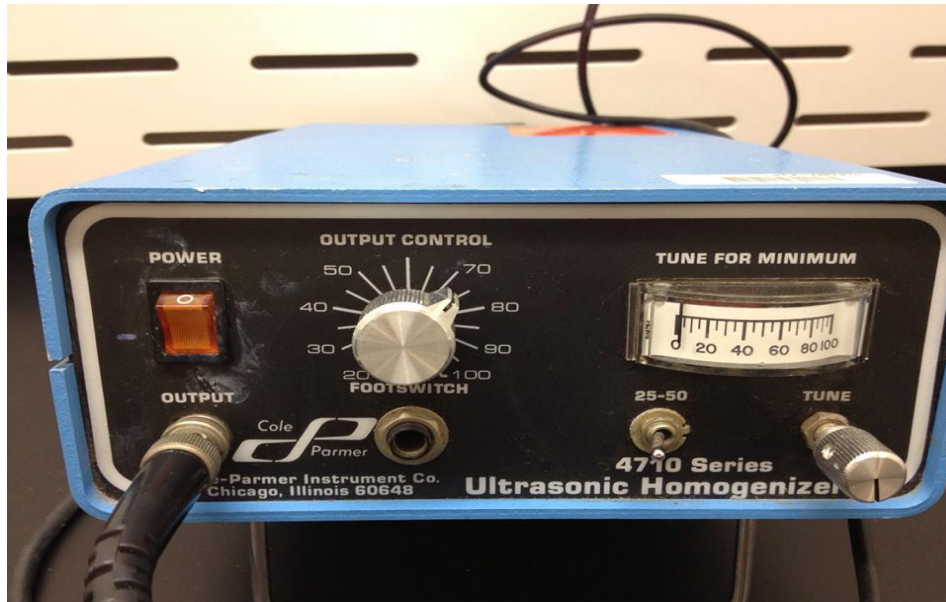
Figure 4: Ultrasound Sonicator and settings used to clean the surfaces of glass microslides.
