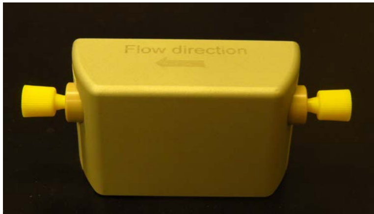
Figure 14: Dolomite microfluidic flow sensor (Part no. 320099) with a measuring range of 0.4-7 \mu\text{L}/\text{min}
