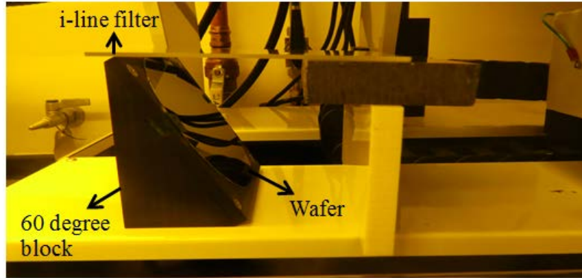
Figure 4: Setup for tilted exposure on the OAI stage
