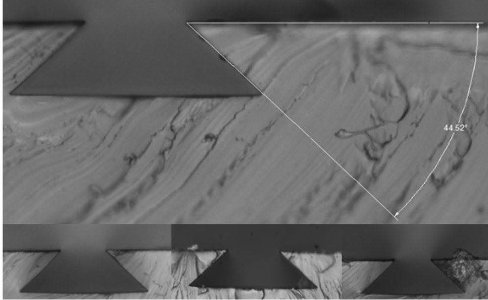
Figure 8: Sidewall angle modulation ( \sim 45^\circ ) using water bath immersion during exposure
