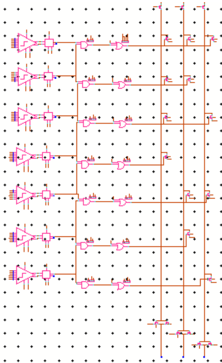
Figure 5-13. Schematic of complete 3-bit Flash with Bubble Correction and ROM encoder
