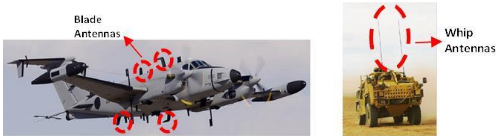
Fig. 1-1 Off- the-shelf Whip and Blade Antennas on Military platforms.
