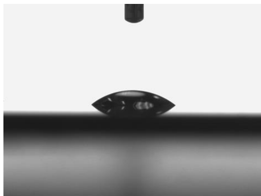
Figure 3.7 The optical image of a water droplet on Imidazole functionalized palladium surface.
