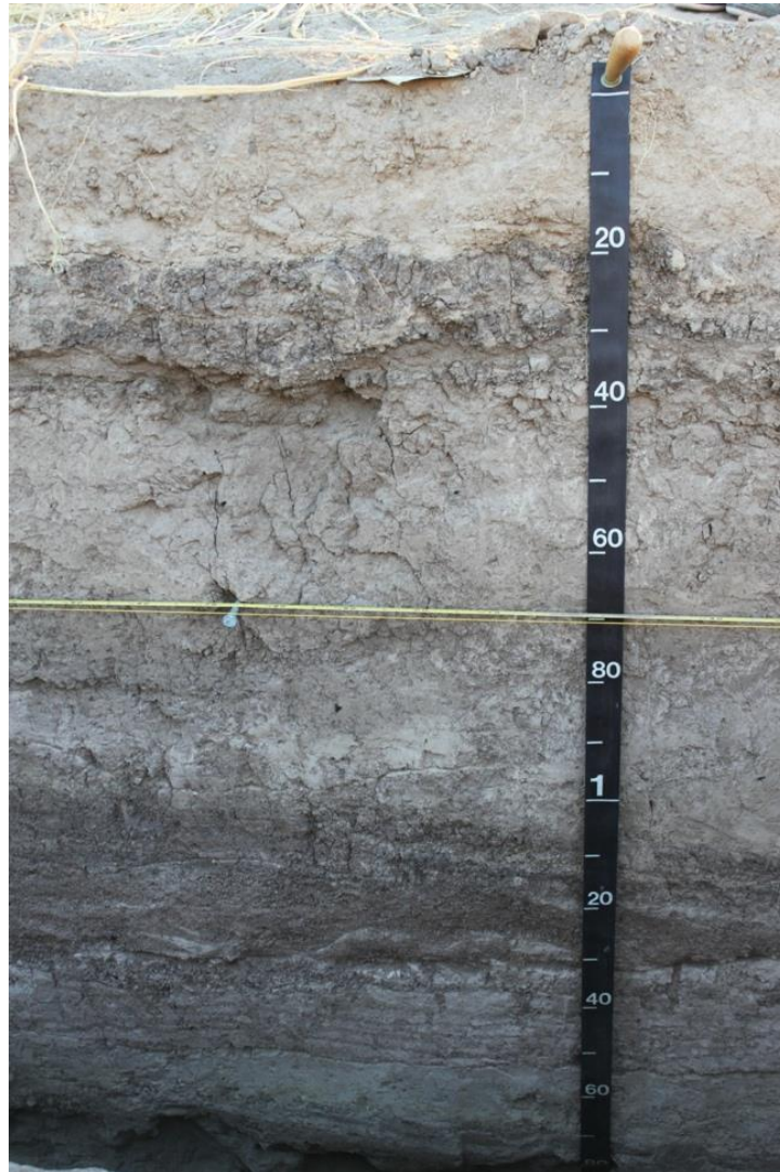
Figure 6.3: Soil Profile of GR 1528. Irrigated field sediments can be observed between 20 and 40 cm on the Measuring Tape.
