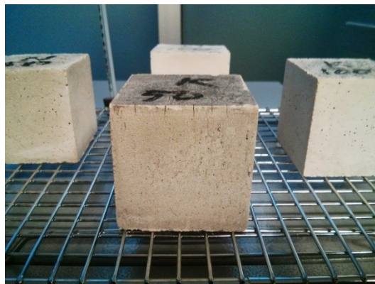
Figure 5-12: Photo of the Vacuum Saturation test samples after removal from the oven at 105°C for 24 h
