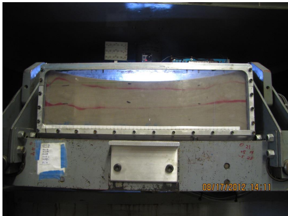
FIG. 3.3. Mounted model ready for centrifuge testing.
