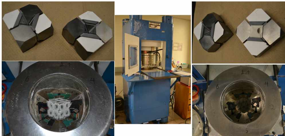
Figure 2.6. Walker 6-8 type multi-anvil apparatus. The eight inner anvils (upper left and right) and the six inner anvils (lower left and right) inside the module. The hydraulic press (middle) is used to apply a hydraulic load.
