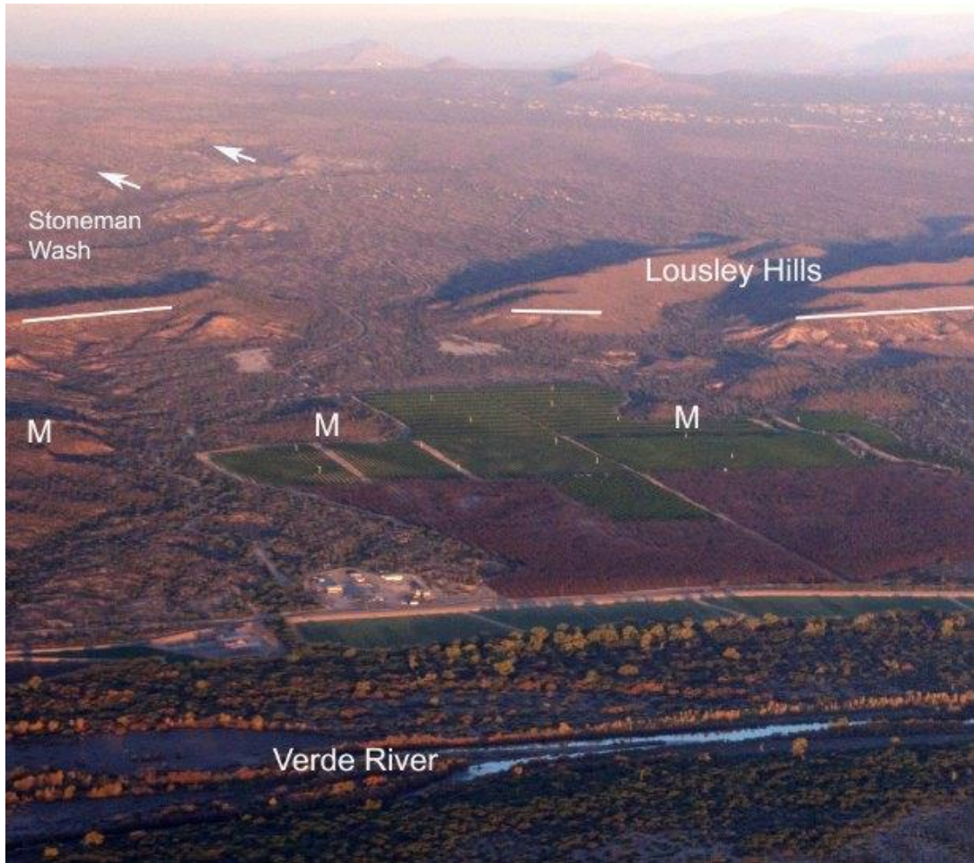
Fig. 4. The lower Verde River displays a complex sequence of events. First, the playa sediments eroded in response to integration of the Salt River (white line). Second, the Lousley Hills gravels deposited — forming a fill terrace. Third, gravels derived from the McDowell Mountains began to accumulate behind the Lousley Hills terrace. Fourth, transverse drainages crossed the Lousley Hills terrace. Fifth, these drainages adjusted to the Mesa River terrace (identified by M), and the eastern McDowell pediment graded to this terrace. Then lowering of the Verde river resulted in a pediment that is undergoing erosion due to knickpoint recession of washes (identified by white arrows).
