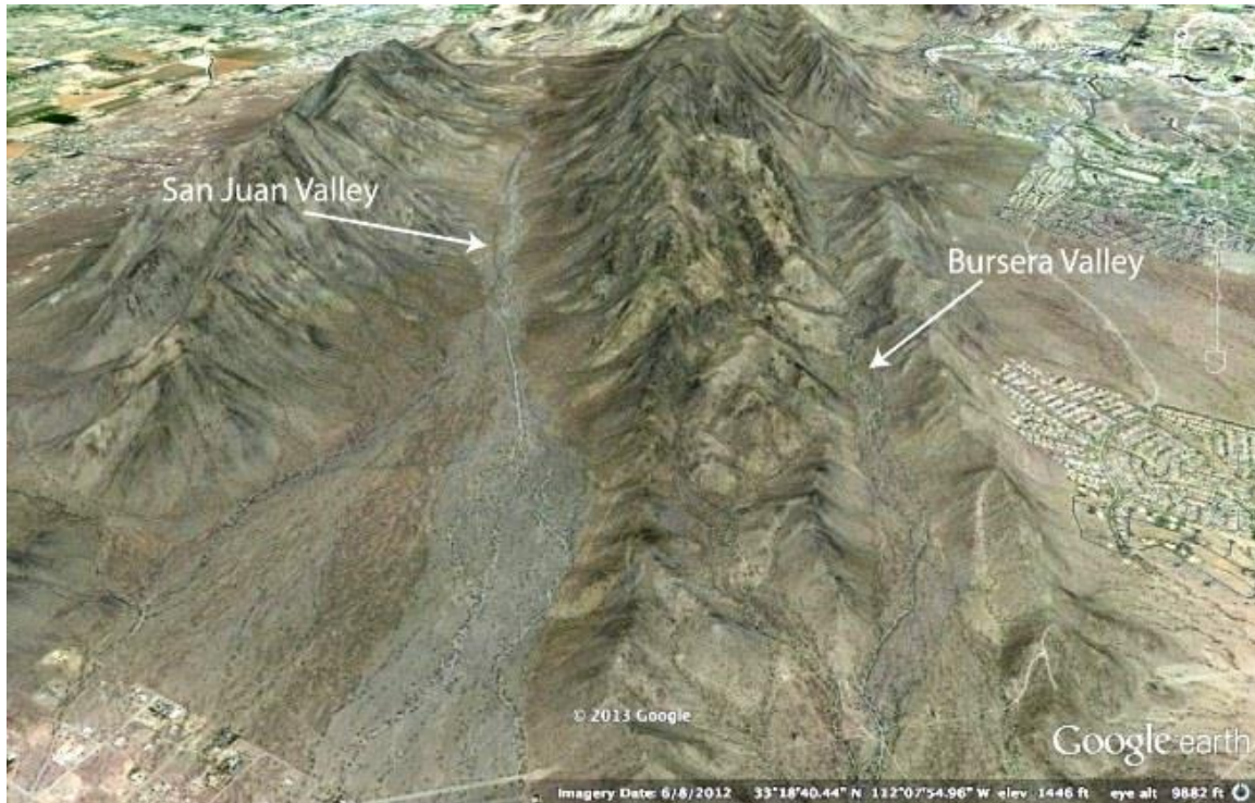
Fig. 15. The San Juan Valley is a classic setting for fan-cut terraces. Alluvial fans emerge from tributary fans on both sides of the axial drainage. San Juan wash has both incised and ‘toe-cut’ the distal reach of these fans resulting in fan-cut terraces. Bursera Canyon has a similar lithology of metamorphic gneiss and small steep basins that generate alluvial fans. This east-looking perspective reveals that the similar gneissic lithologies and a similar geologic setting to an adjacent canyon would be one piece of evidence in favor of a fan-cut interpretation. The image follows Google Earth usage guidelines [ http://www.google.com/permissions/geoguidelines.html ].
