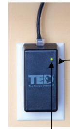
Green Light on the front and side of Gateway should always be blinking consistently
