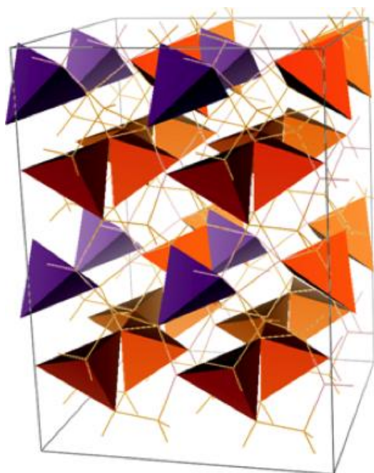
Figure 18. Calculated ordered structure of an AlAs_{0.25}P_{0.75}Si_3 alloy in which the AlPSi_3 and AlAsSi_3 building units are shown as orange and purple tetrahedra, respectively (DFT estimate a=5.484 \text{ \AA} ).
