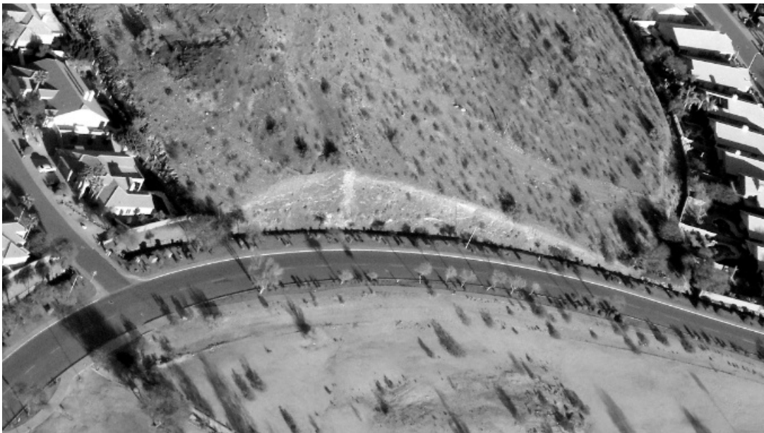
Figure 4. Oblique aerial photograph showing the context of the Marketplace study site, randomly selected for this study. The bedrock fractures filled with carbonate can even be seen as bright lines from a flying altitude of about 1000 m above the surface.
