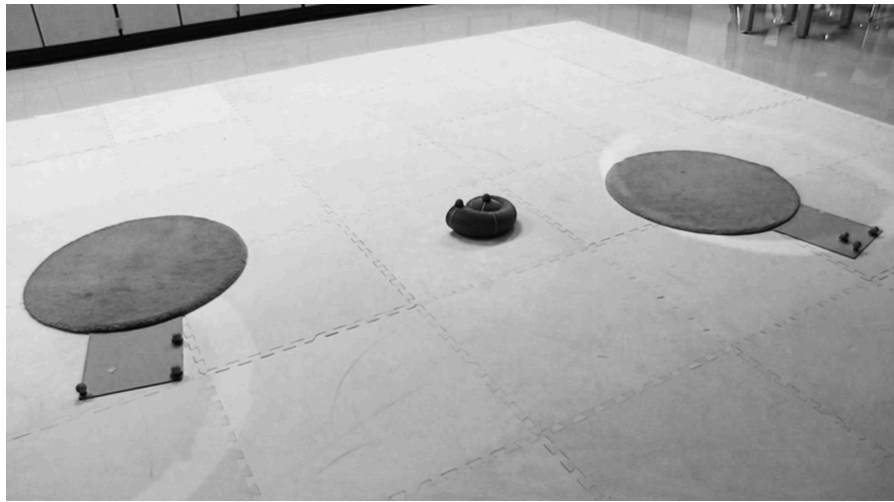
Figure 45. Tan circle rugs with cardboard wings. Rugs, approximately 2.5 feet in diameter, with cardboard wings serving as tracked objects for placing Velcro balls with reflective tape. At the center of the floor is a custom-built seashell shaped object that contains a wireless microphone unit. This object is also being tracked via motion capture and has two Velcro balls placed on top.
