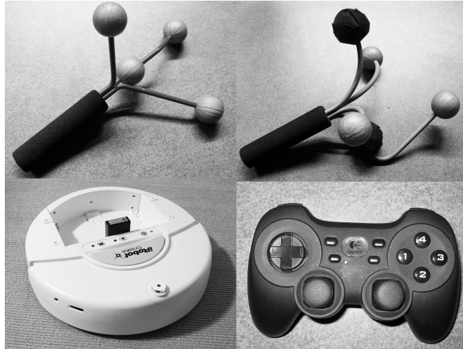
Figure 42. Trackable objects and peripherals. Two wands (top two photos) have infrared marker balls mounted in unique geometries to allow the Optitrack cameras to distinguish between them. Motion tracking software calculates each object's position and rotation data, which is then passed across the local network via UDP. Infrared markers are placed on the iRobot (bottom left), which can be controlled using Bluetooth. The Logitech Gamepad (bottom right) can be used to change SMALLab scenes and feedback.
