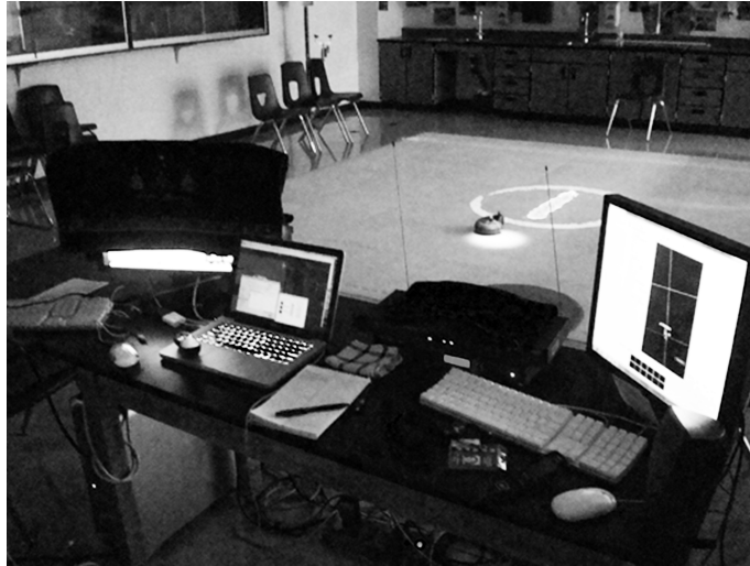
Figure 44. SMALLab monitoring station. The station is set to the side of the SMALLab space, to allow researchers and designers to monitor the system and make changes.
