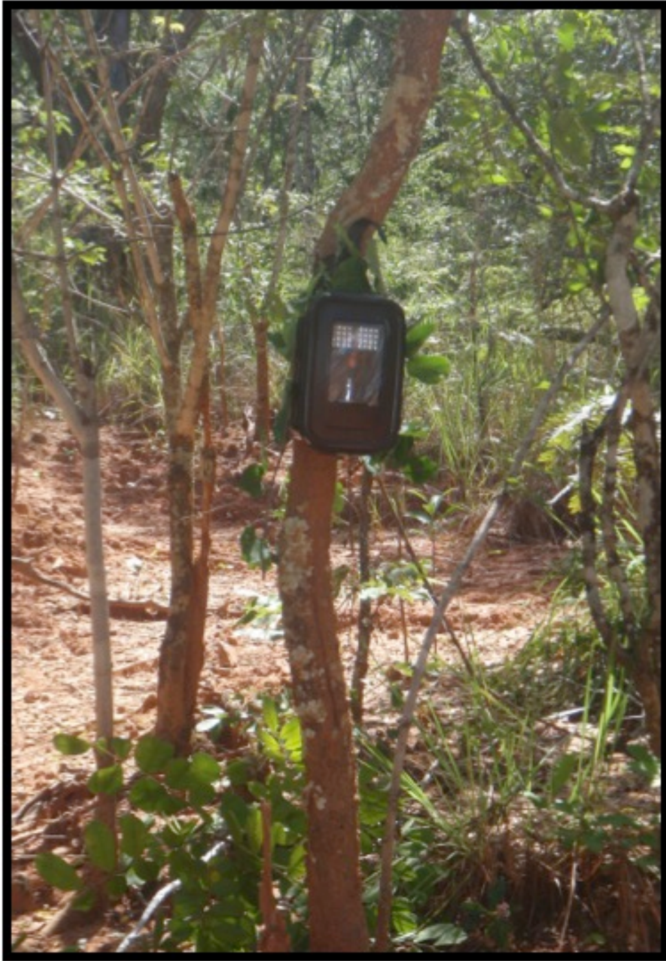
Figure 4-3. Setup of digital camera trap (camera is encased in plastic container for weather protection).
