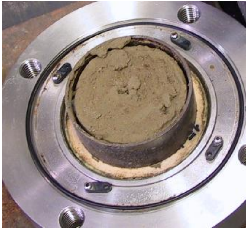
Figure A.13. Slurry Specimen of San Antonio on High Air Entry Ceramic Stone of SWCC Cell Equilibrated at 50kPa Suction under Token Load
