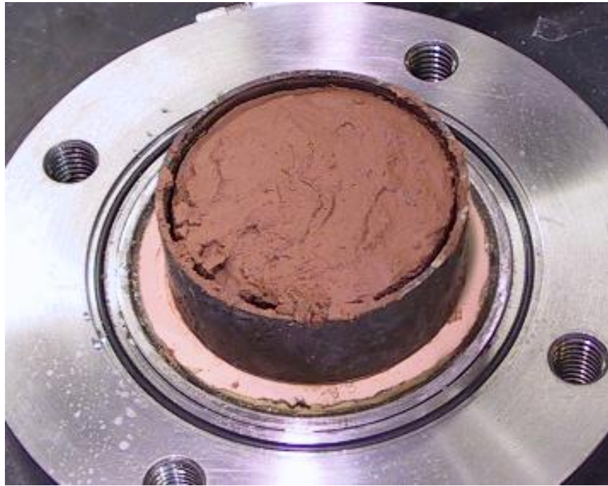
Figure A.1. Slurry Specimen of Anthem on High Air Entry Ceramic Stone of SWCC Cell Equilibrated at 25kPa Suction under Token Load
