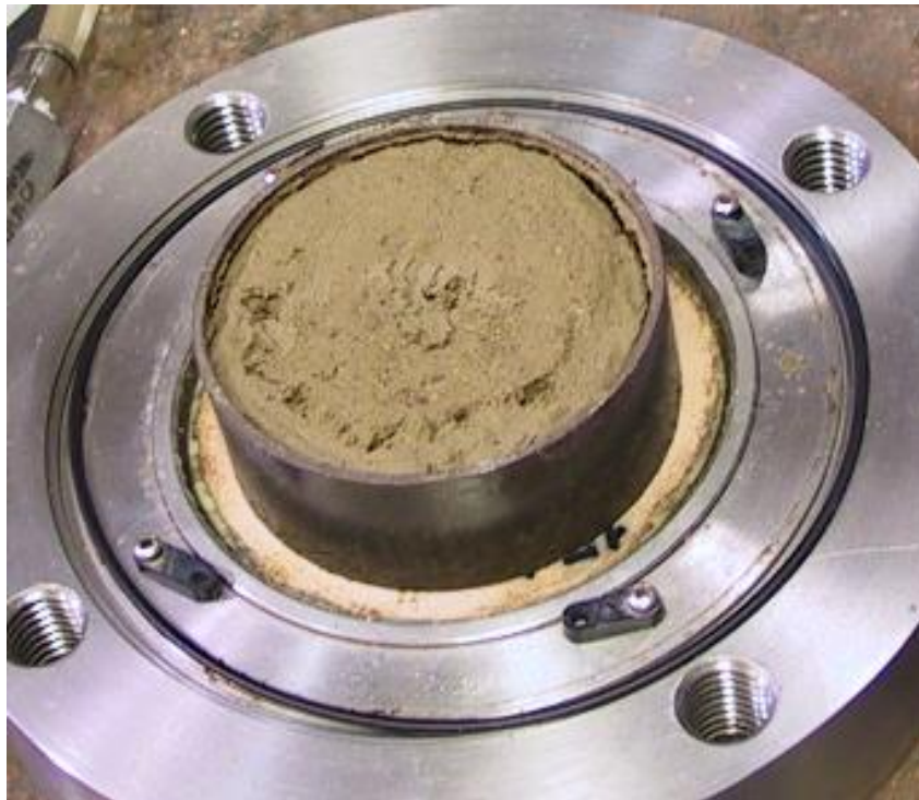
Figure A.12. Slurry Specimen of San Antonio on High Air Entry Ceramic Stone of SWCC Cell Equilibrated at 25kPa Suction under Token Load
