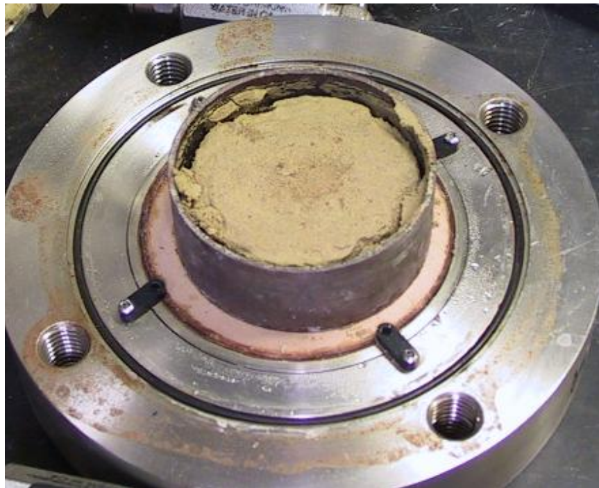
Figure A.8. Slurry Specimen of Colorado on High Air Entry Ceramic Stone of SWCC Cell Equilibrated at 50kPa Suction under Token Load
