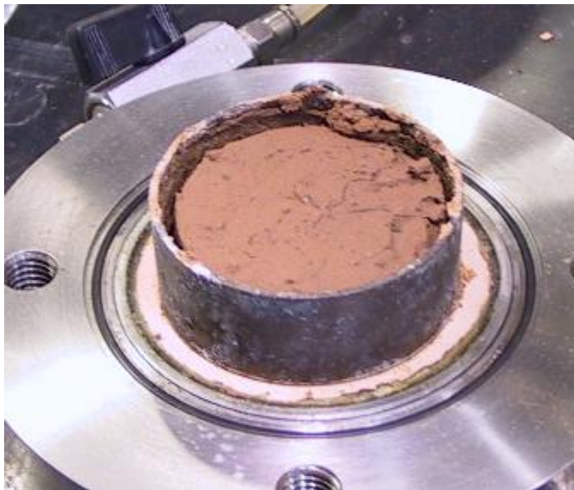
Figure A.4. Slurry Specimen of Anthem on High Air Entry Ceramic Stone of SWCC Cell Equilibrated at 200kPa Suction under Token Load
