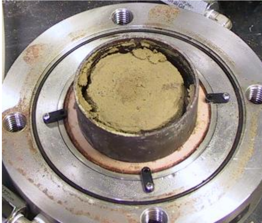
Figure A.11. Slurry Specimen of Colorado on High Air Entry Ceramic Stone of SWCC Cell Equilibrated at 400kPa Suction under Token Load
