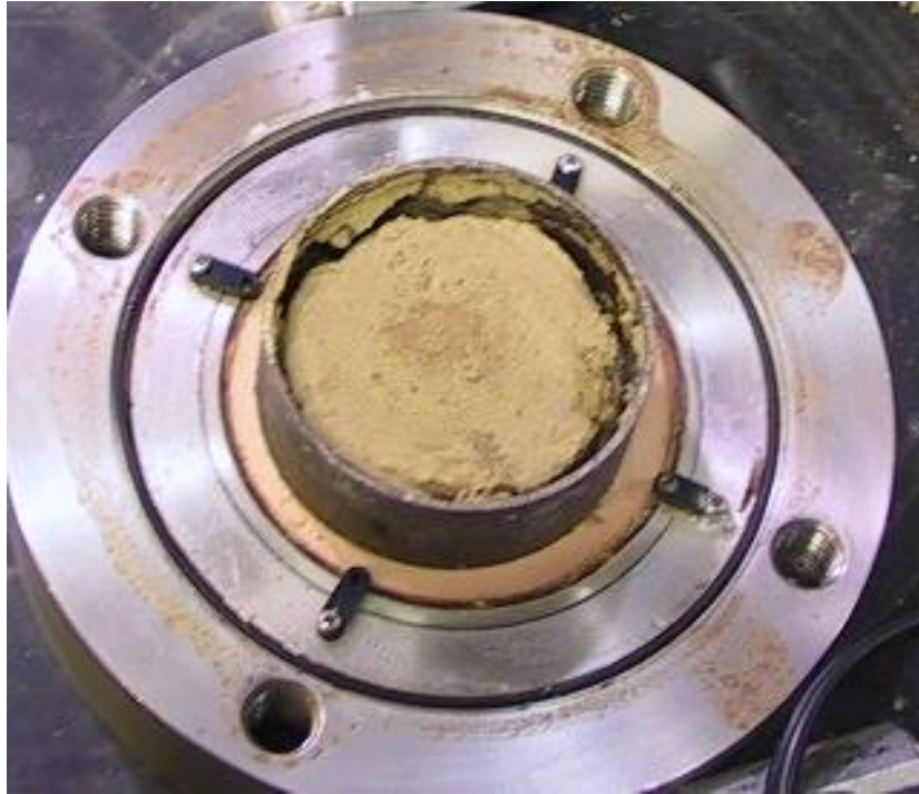
Figure A.9. Slurry Specimen of Colorado on High Air Entry Ceramic Stone of SWCC Cell Equilibrated at 100kPa Suction under Token Load
