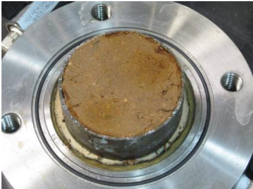
Figure 3.67. Anthem specimen equilibrated at suction of 1330kPa under net normal stress of 53kPa (46% Swell Pressure). Note the minimal radial shrinkage in the specimen, although there is some vertical displacement
