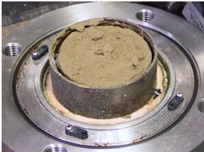
Figure A.14. Slurry Specimen of San Antonio on High Air Entry Ceramic Stone of SWCC Cell Equilibrated at 100kPa Suction under Token Load
