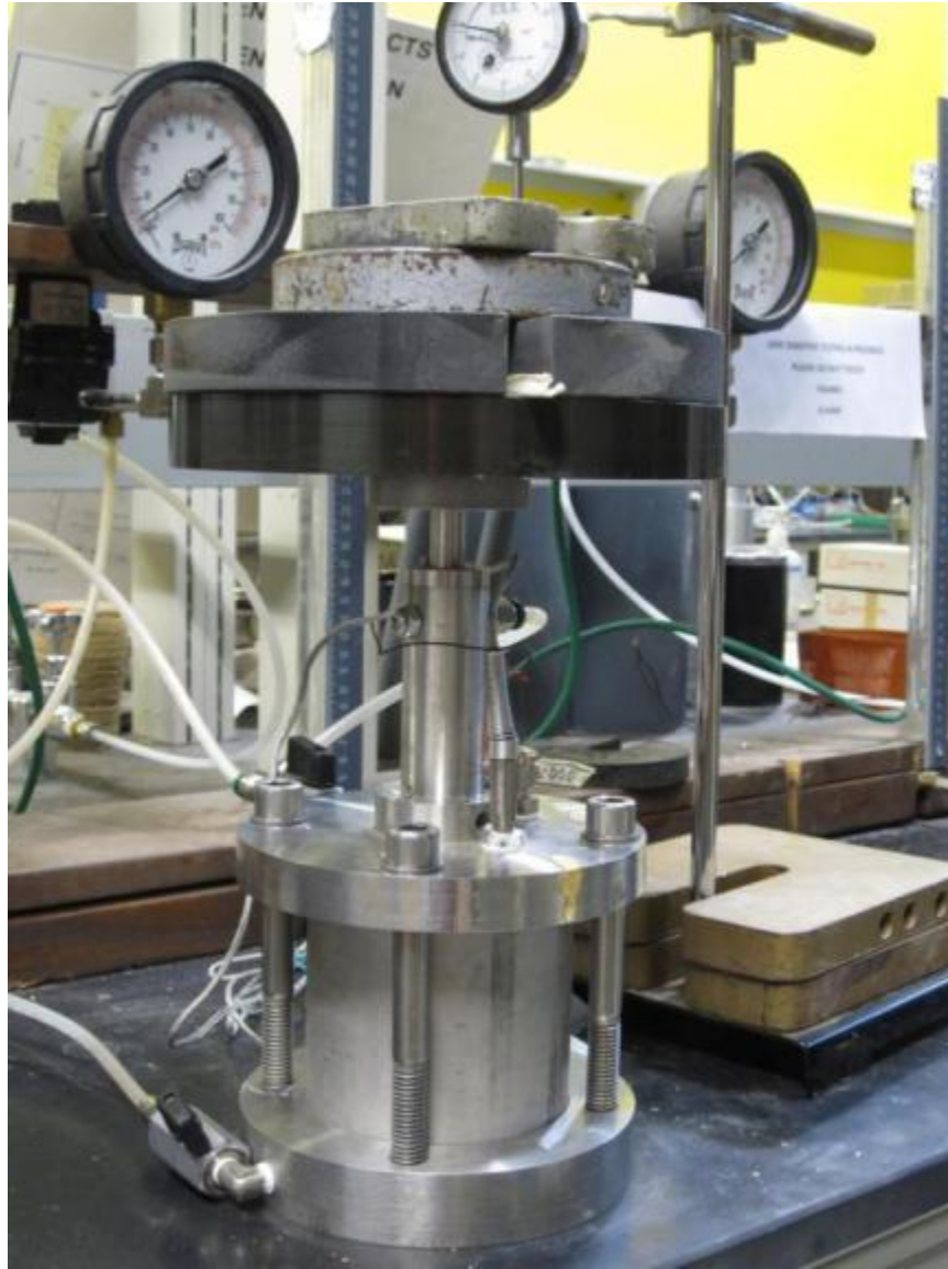
Figure A.27. Application of Net Normal Pressure to Specimens and Monitoring Vertical displacement Using Dial Gauges
