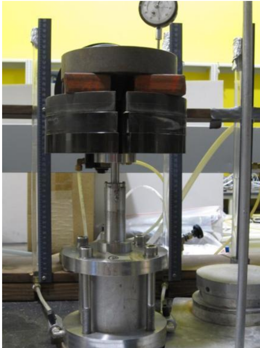
Figure A.28. Application of Net Normal Pressure to Specimens and Monitoring Vertical displacement Using Dial Gauges
