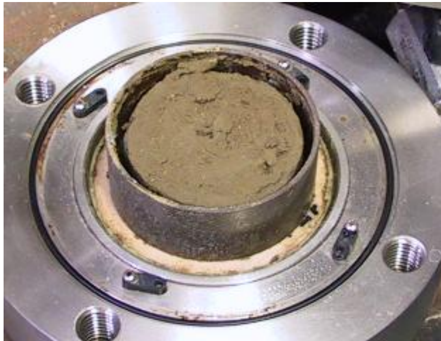
Figure A.16. Slurry Specimen of San Antonio on High Air Entry Ceramic Stone of SWCC Cell Equilibrated at 400kPa Suction under Token Load
