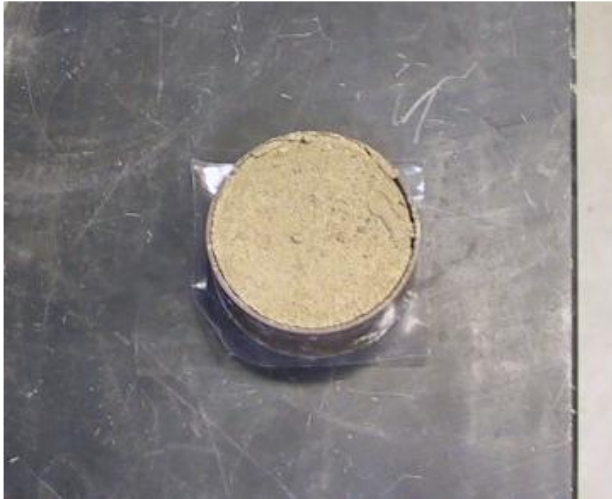
Figure A.22. Compacted Specimen of Colorado Equilibrated at 400kPa Suction under Seating Load
