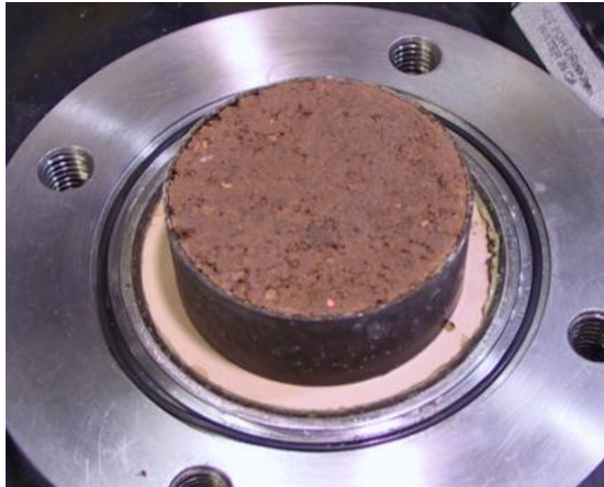
Figure A.17. Compacted Specimen of Anthem on High Air Entry Ceramic Stone of SWCC Cell Equilibrated at 100kPa Suction under Seating Load
