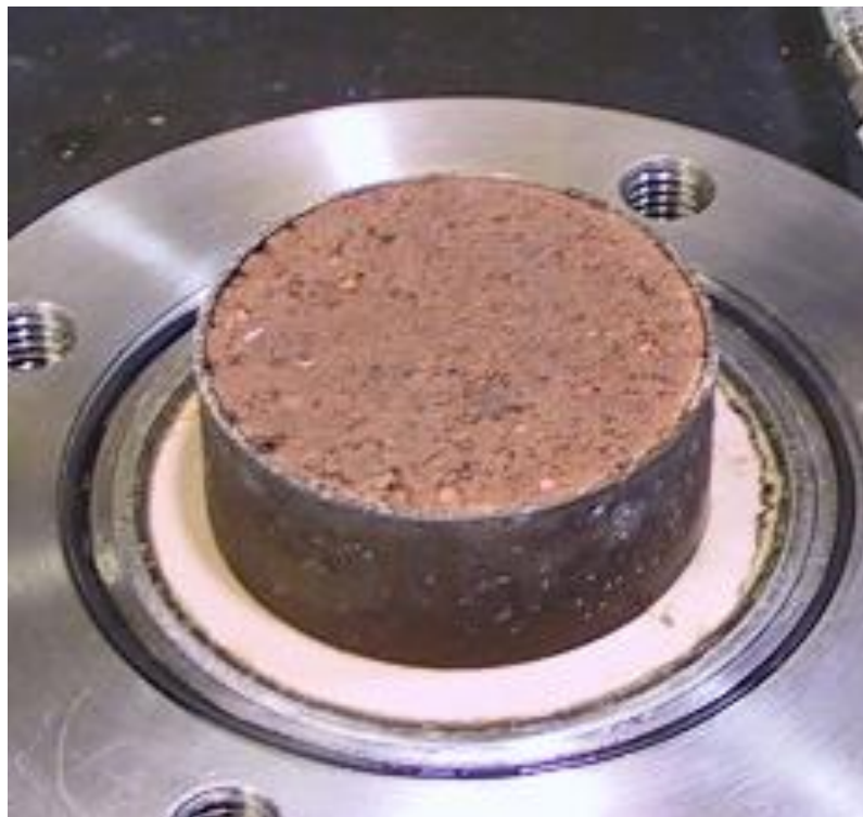
Figure A.18. Compacted Specimen of Anthem on High Air Entry Ceramic Stone of SWCC Cell Equilibrated at 400kPa Suction under Seating Load
