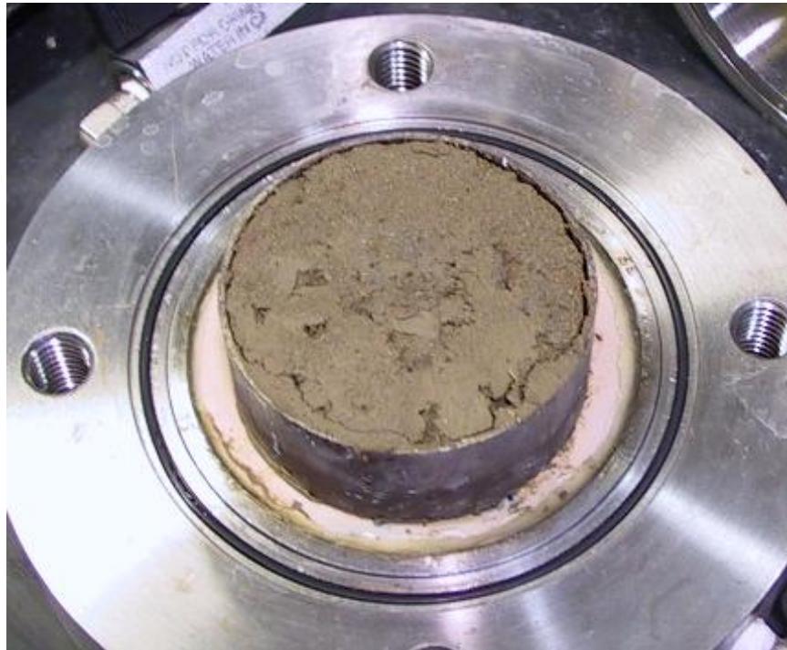
Figure A.23. Compacted Specimen of San Antonio on High Air Entry Ceramic Stone of SWCC Cell Equilibrated at 400kPa Suction under Seating Load
