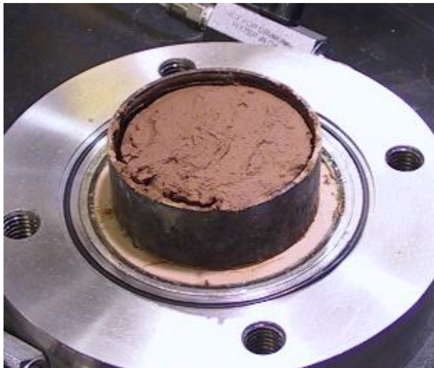
Figure A.2. Slurry Specimen of Anthem on High Air Entry Ceramic Stone of SWCC Cell Equilibrated at 50kPa Suction under Token Load
