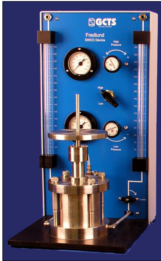
Figure 1.1. Oedometer pressure plate device, SWC-150 (GCTS, 2004)
