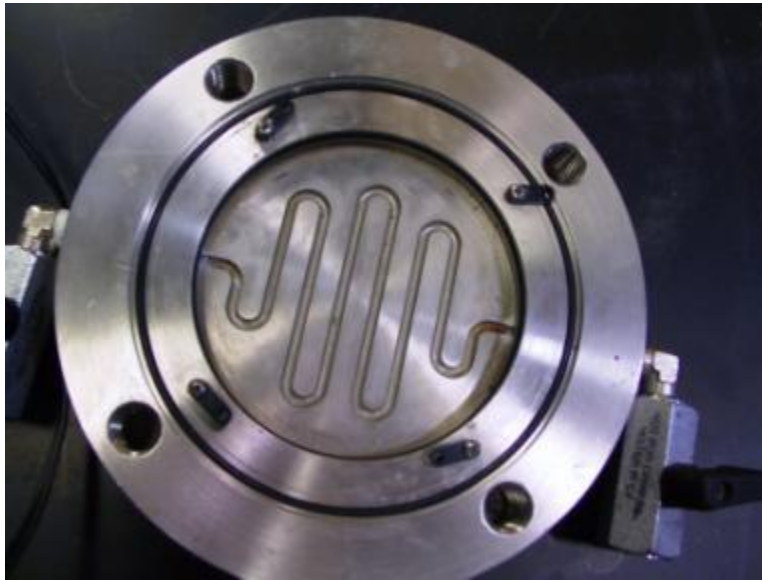
Figure 3.3. SWC-150 cell bottom plate (base) with grooved channel (Abbaszadeh, 2011)
