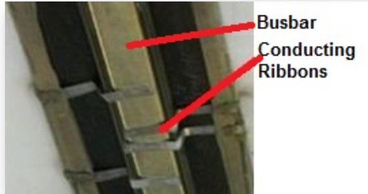
Figure 24 – Module Power Conducting Ribbons Connected To Busbar
