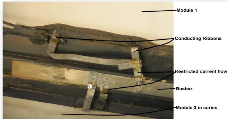
Figure 26 – Example of Incorrect Ribbon Connection
