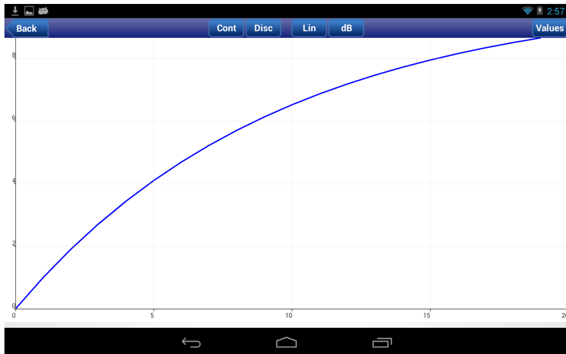
Fig 3.8. Impulse response of a filter with H(Z) = \frac{(z^{-1})}{(1-9z^{-1})}
