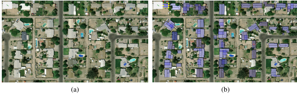
Figure 3.18: Evaluation of gable roof shape detection by our algorithm; (a) aerial image with 40 gable roofs; (b) parametric models identified, placed over the original image
