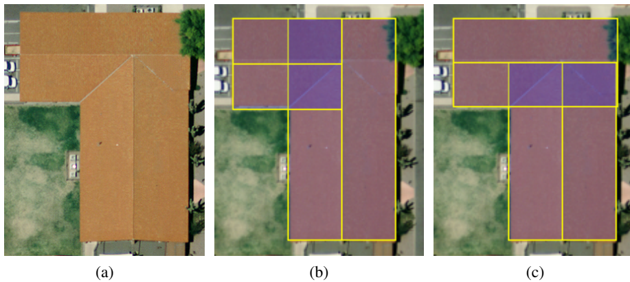
Figure 3.11: A case where algorithm fails to detect the correct building blocks; (a) reference building; (b) incorrect configuration chosen by our algorithm to represent building based on largest rectangle first; (c) manually chosen correct configuration
