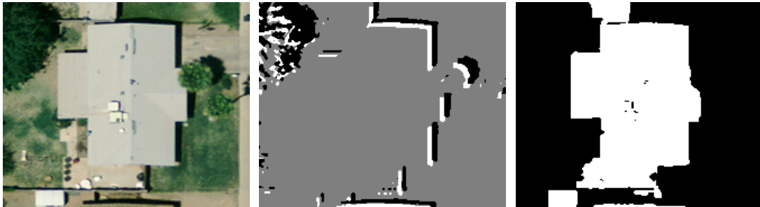
Figure 2.6: Example of successful roof detection when shadow has gaps (notice tree obstructing shadow of building); (a) roof image; (b) initial foreground / background assignment; (c) result of grabcut on (b)
