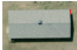
Figure 2.11: Image showing overhang of shadow (notice the red line marked between the corner of roof and point from where shadow starts)
