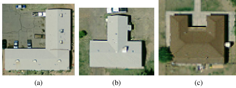
Figure 3.5: Complex rectilinear roofs; (a) 'L' shaped; (b) 'T' shaped; (c) 'U' shaped
