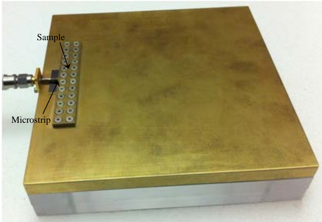
Fig. 36. Microstrip Permeameter designed to fit thin film ferrite samples.
