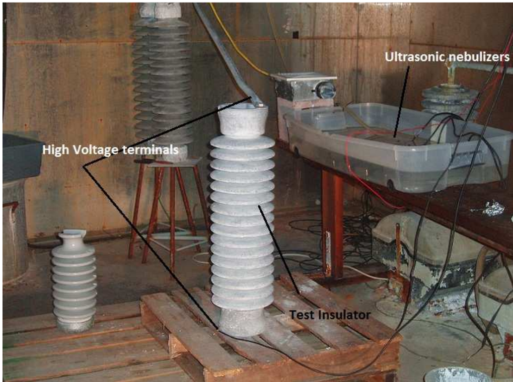
Figure 4.2 Experimental set-up in the fog chamber
