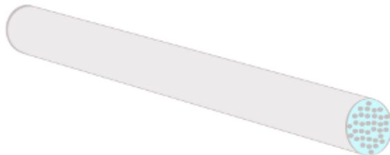
Fig. 2-6 Third Suggested Option for Waveguiding Structure, Cylinder of Effective Media Constructed from Colloidal Spheres
