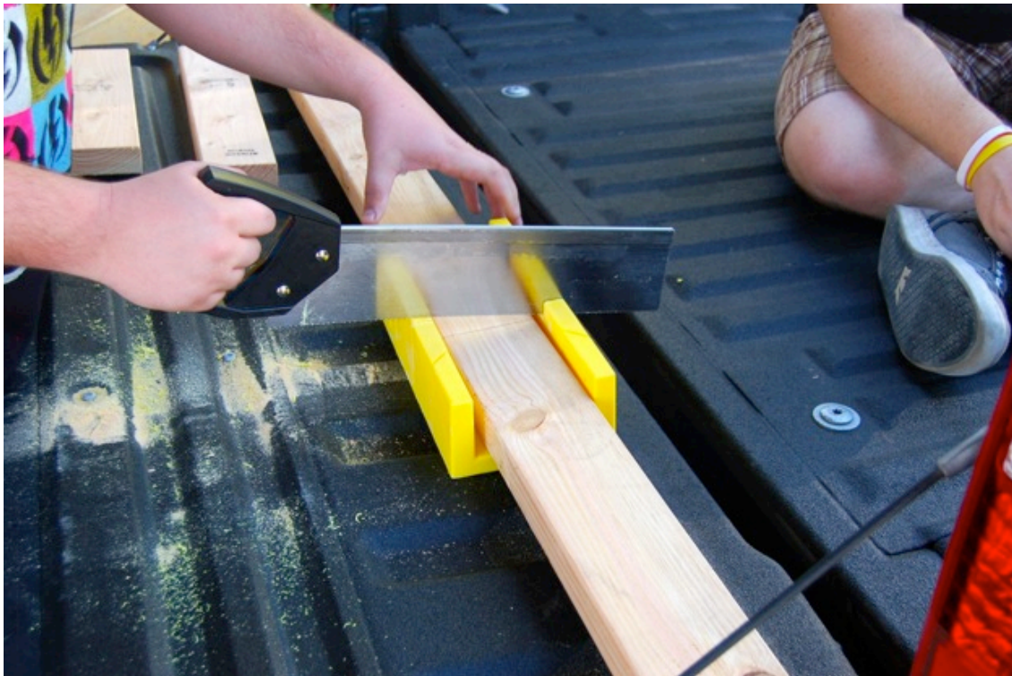
Figure 5. Miter Box (supplied) with short sides
