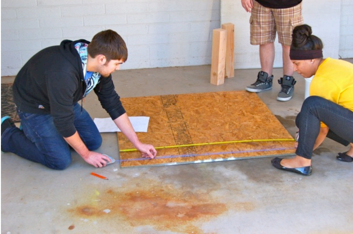
Figure 12. Team using chalk line to make long straight markings on plywood
