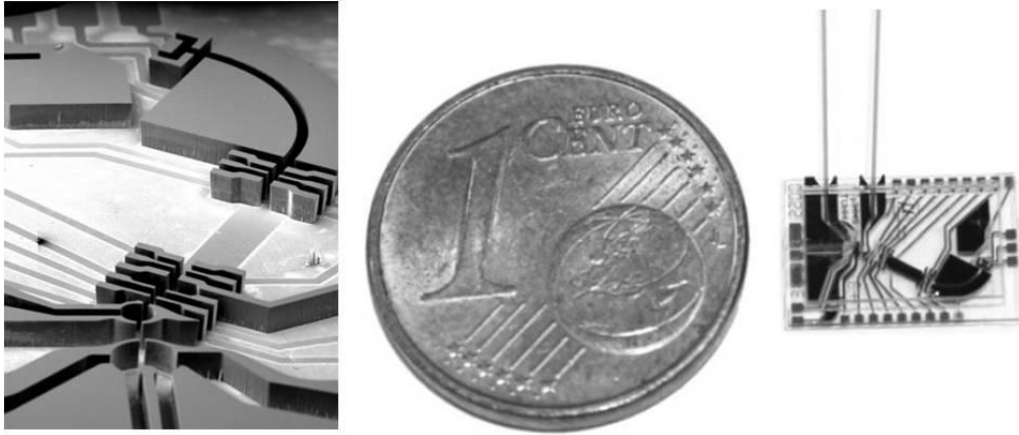
Figure 1.10: A fully integrated time-of-flight mass spectrometer. (left) A scanning electron micrograph showing the mass filter. (right) The packaged mass spectrometer shown next to a penny for scale (Wapelhorst et al. 2007).
