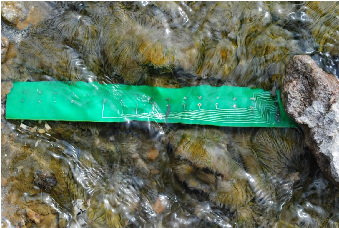
Figure 5.2: Photograph of the microbial mat community found in the alkaline outflow channel. The temperature array is 2.4 cm by 18.5 cm.
