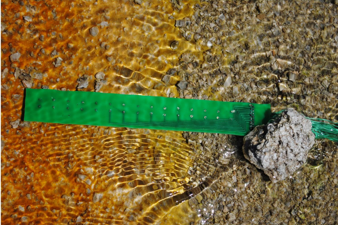
Figure 3.35: Close-up photograph of the temperature array in the outflow channel of a geyser in Imperial Geyser Basin. The length of the array is 18.5 cm for scale.
