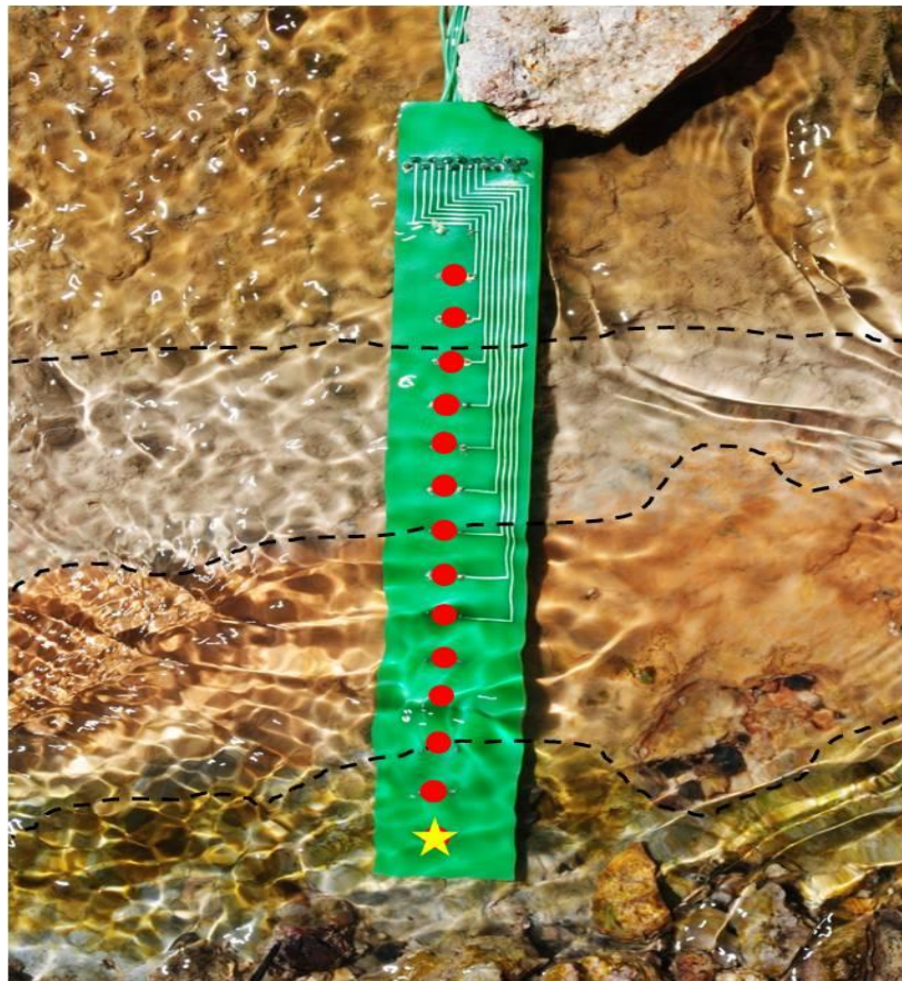
Figure 5.5: Photograph of an 18.5 cm long temperature array placed across the microbial striping zone with dashed lines outlining four distinct color regions. The yellow star marks the zero position in the temperature plot.
