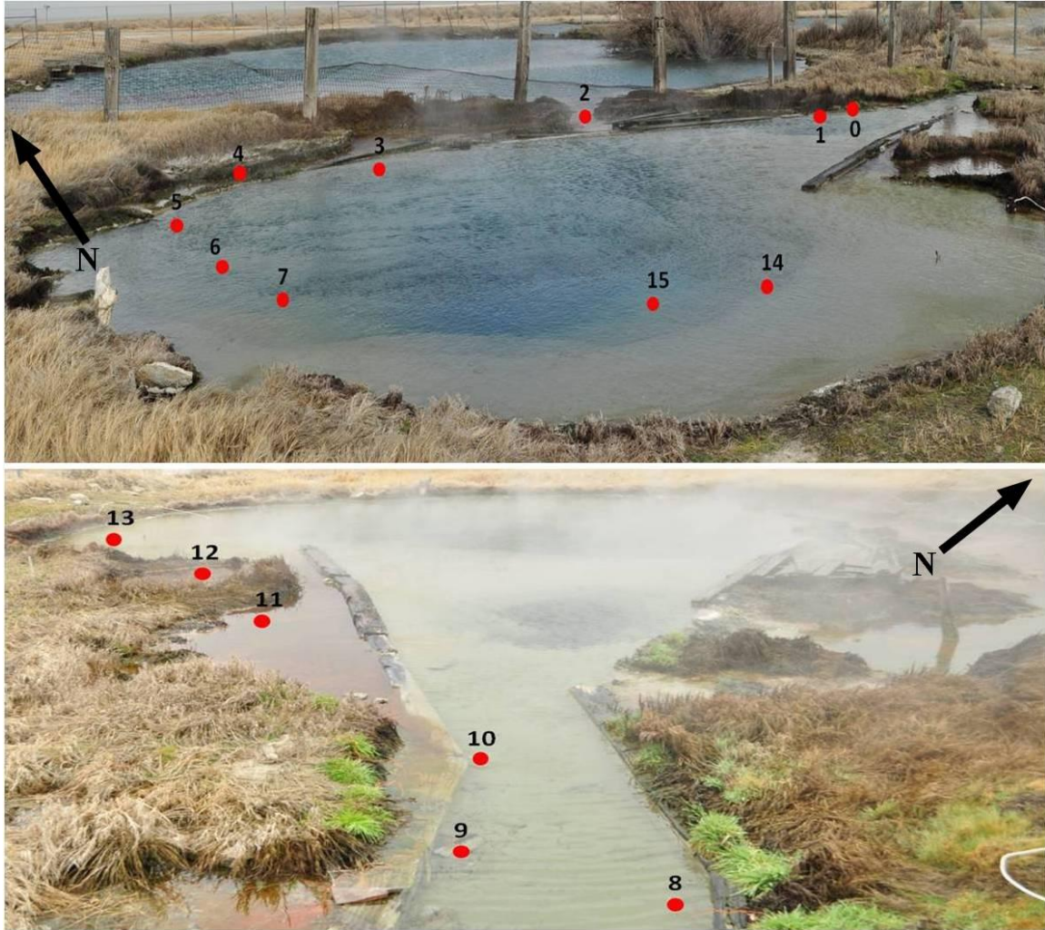
Figure 3.39: Photographs of Great Boiling Spring hot spring (GBS), Gerlach, NV, from two different directions where the first long-term monitoring station was set up. The red dots represent the locations where 16 individual RTDs were placed in the hot spring. The numbers correspond to the sensor numbers provided in the following plot. Arrows pointing north are provided for orientation. The GBS pool is ~6.5 m in diameter.
