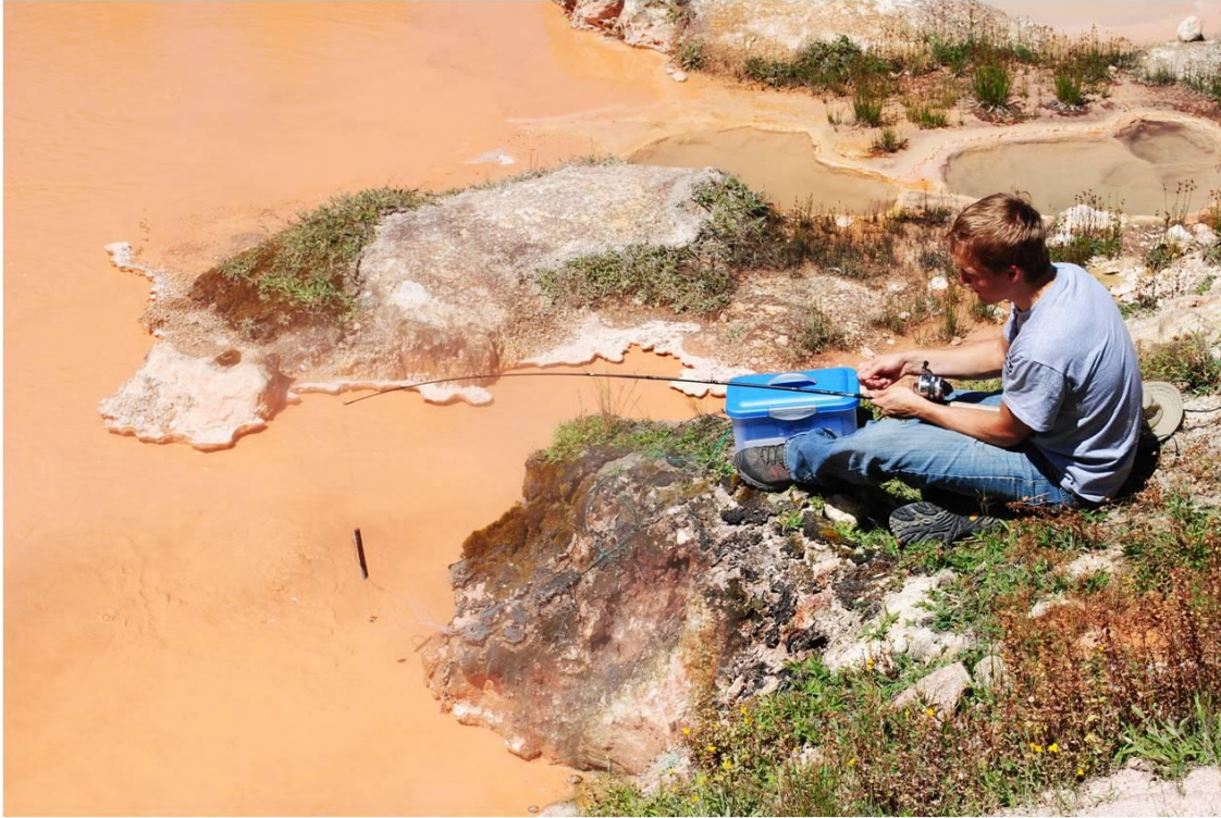
Figure 3.32: Photograph of a temperature array connected to a fishing pole in order to measure temperature at depth in a hot spring source pool.
