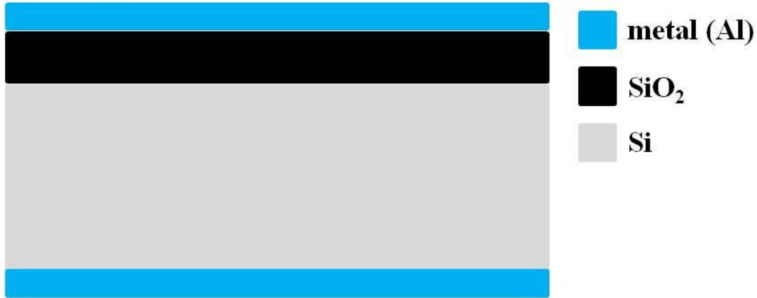
Figure 2.2: Schematic cross-section drawing of a MOS capacitor. Most commonly, a layer of silicon dioxide thermally grown on a layer of silicon is sandwiched between two aluminum electrodes.
