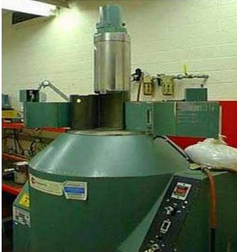
Figure 2.5: Radiation testing equipment in Professor Holbert's laboratory. Devices are exposed to 1.2 MeV photons from a ^{60}\text{Co} source in the belly of the lead-shielded machine.
