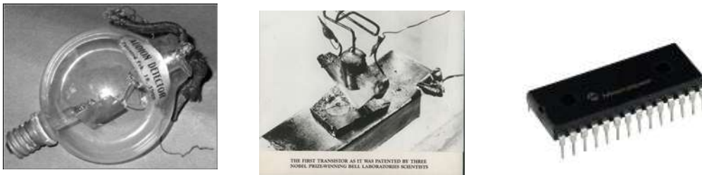
Figure1.1. Evolution of modern day ICs from vacuum tubes.
