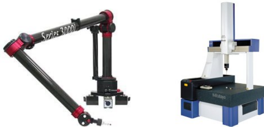
Figure 1.1. Typical types of CMM machines: Portable CMM (left) and gantry type (right)
