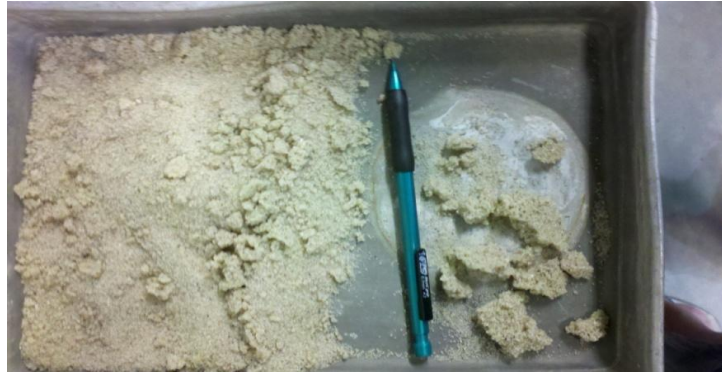
Figure 26- Example of weakly cemented chunks of sand observed in Sand Columns 3 through 6 after rinsing and drying (Sand Column 5 shown).
