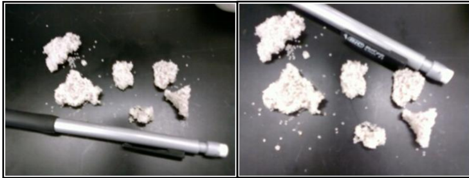
Figure 6 -Small pieces of loosely cemented sand grains from static sand column experiments containing \text{CaCl}_2 with L-glutamic acid as an electron donor.
