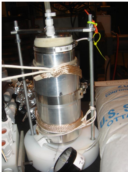
Figure 10- The fully assembled sand column bolted to the base plate.
