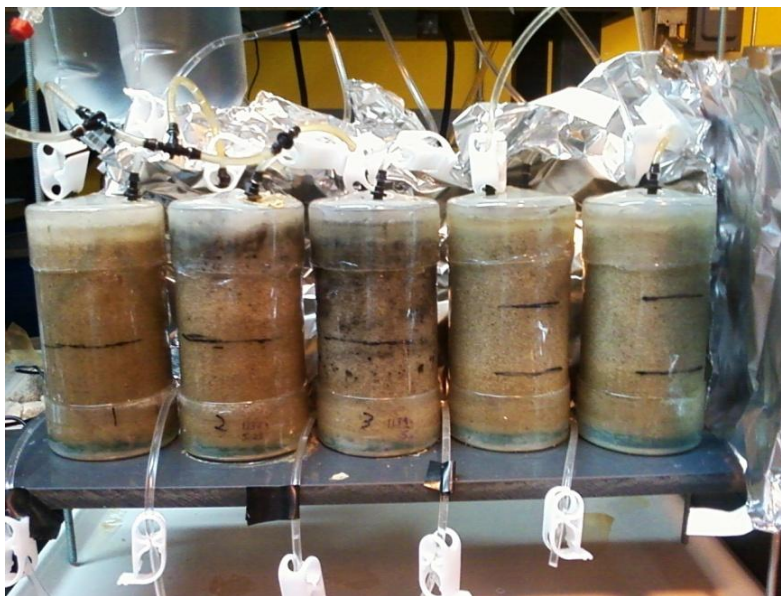
Figure 12a- Five acrylic sand columns are filled and sitting on a PVC platform. Some of the columns were interconnected depending on the column treatment.
