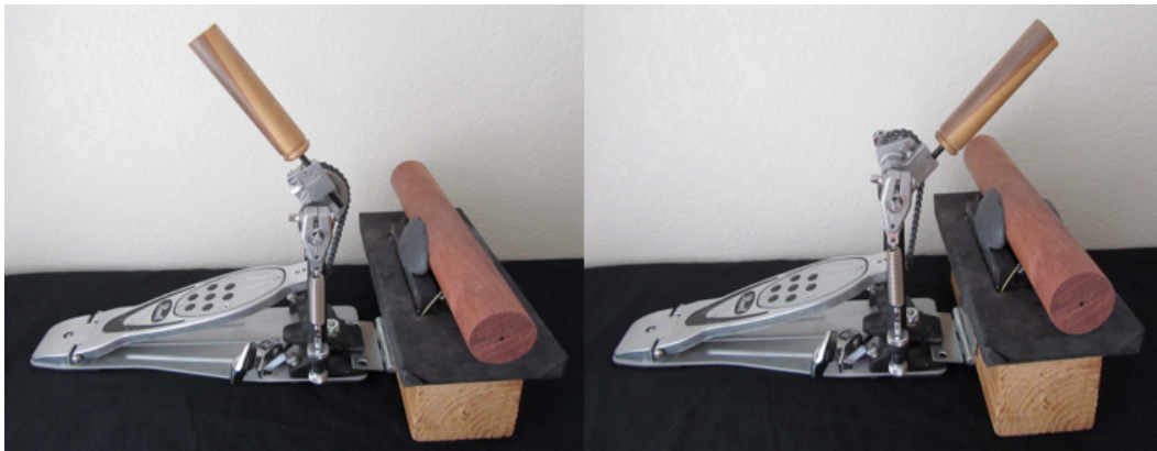
Figure 5.5 Clave beater angle adjustment 43
