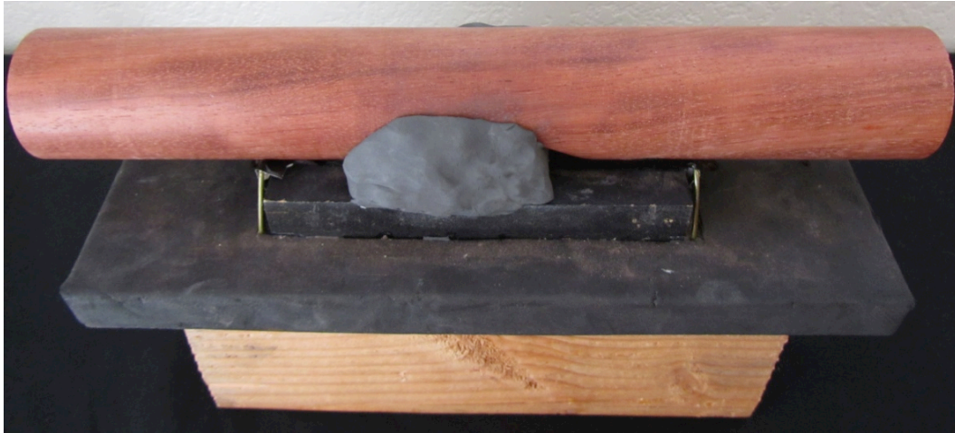
Figure 5.3 Clave mounting system with modeling clay 41
