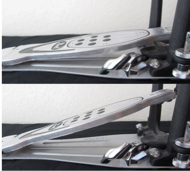
Figure 3.7. Pedal footboard height adjustment
