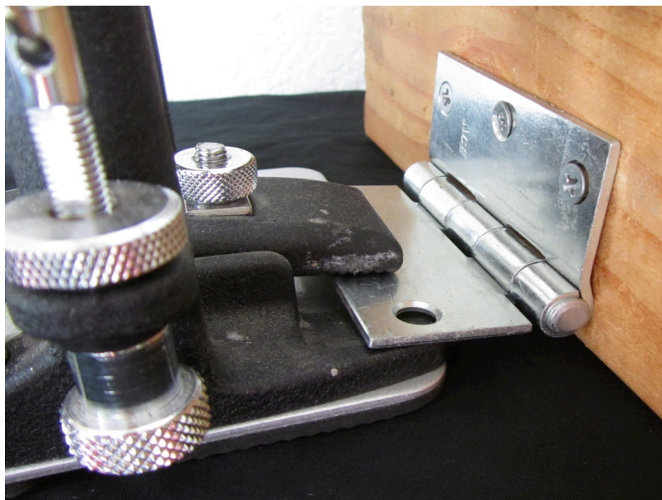
Figure 5.4 Hinged mount on foot-pedaled clavichord 42
