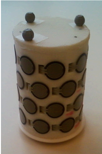
Figure 37. Picture of the cylinder object. This object can be used to do reach and grasp tasks or reach to grasp and transport tasks.
