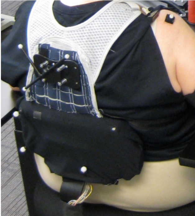
Figure 9. Revised marker configuration for the right shoulder and torso.
