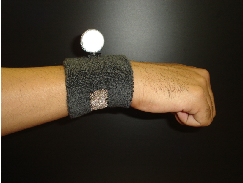
Figure 24. Wristband with reflective motion capture marker and conductive cloth used for rest position contact switch.
