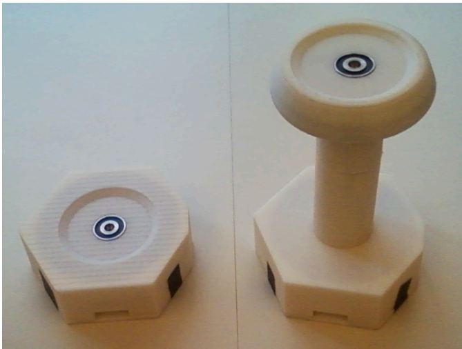
Figure 38. On and off table receptacles for the transportable Cylinder object, showing the electromagnet that bonds the object to the receptacle, providing a stable target
