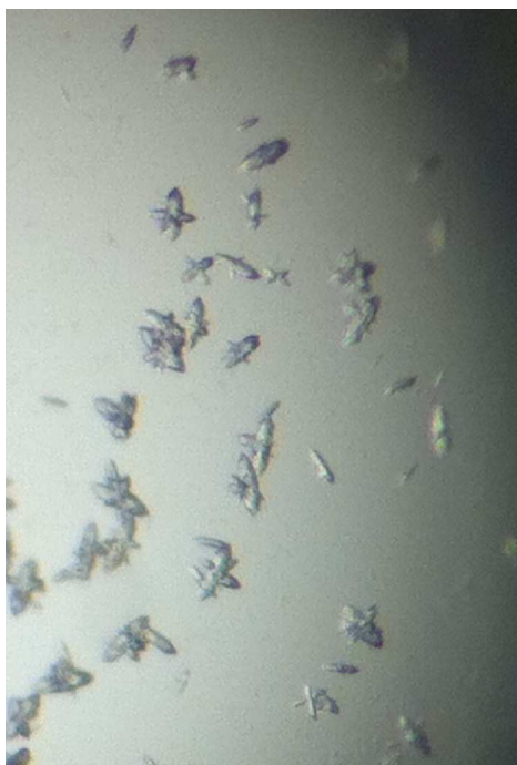
Figure 2.8- Crystallization of N45-Gemin2 N45-Gemin2 was crystallized in 0.1M HEPES pH 7.5, 1.5M lithium sulfate using the hanging drop method. Crystals were approximately 2 µm in size.
