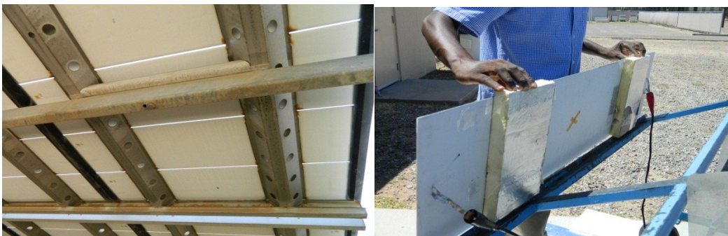
Figure 4.16 Hot area cell effects on modules back side (Left: In the field. Right: Simulated in the lab)
