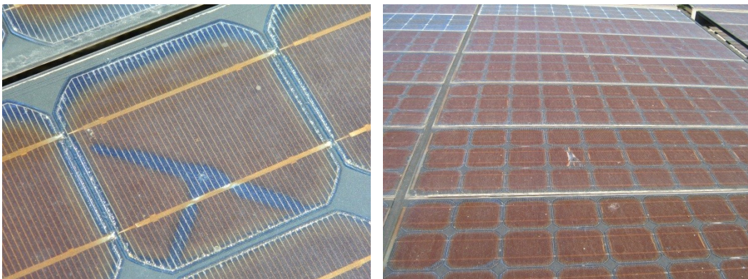
Figure 4.21 Left: cracks on module interconnect. Right: breakages observed in module interconnects in the PV array
