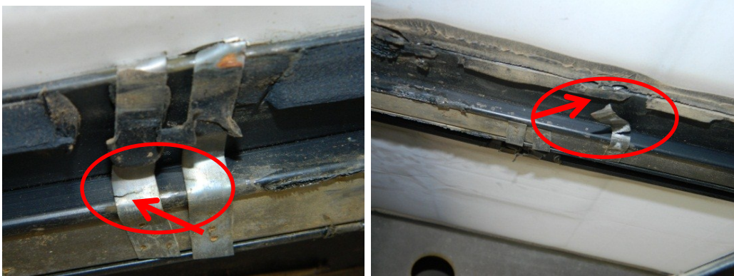
Figure 4.21 Left: cracks on module interconnect. Right: breakages observed in module interconnects in the PV array
