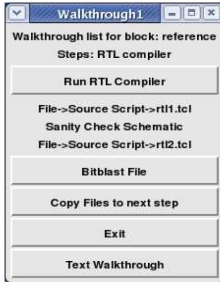
Fig 4.2. Walkthrough GUI for the synthesis step. Actions and scripts that can be run by the GUI itself are presented as buttons, while actions that must be taken in the tool are presented as a list.
