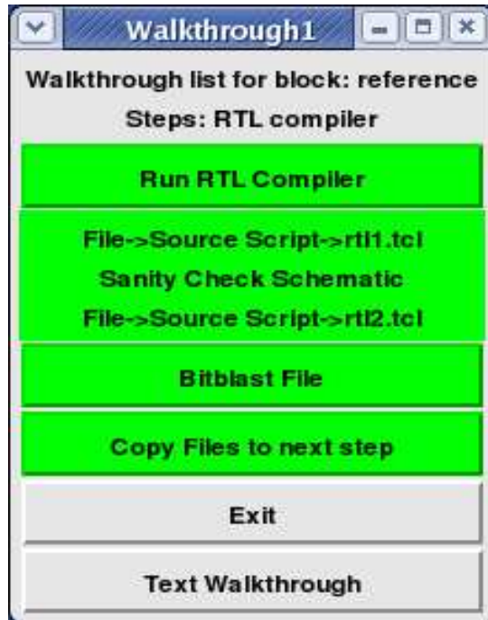
Fig. 4.3. GUI status indicator for the synthesis step. Since each button before the “Exit” button has been pressed, the steps have had their background changed to green.
